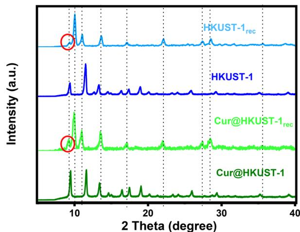
Fig. 10 XRD patterns of Cur@HKUST-1, HKUST-1, Cur@HKUST-1<sub>REC</sub> and HKUST-1<sub>REC</sub>. The plane (2 2 0) attributed to HKUST-1 was highlighted with a red circle.
