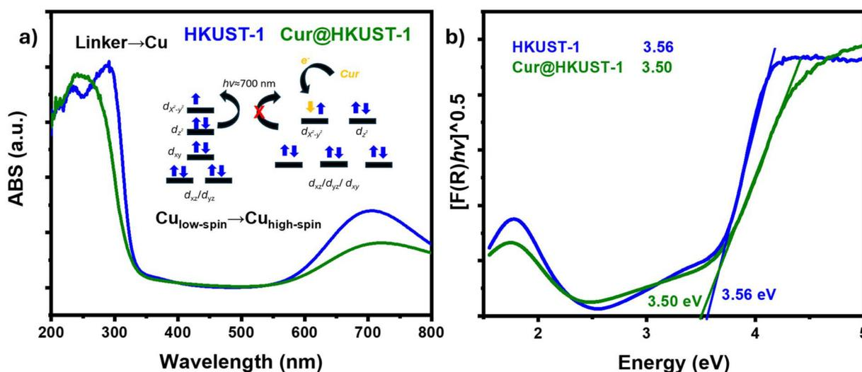
**Fig. 4** For HKUST-1 (blue line) and Cur@HKUST-1 (green line): (a) UV-vis spectra, and energy orbitals diagram indicating comparative electronic promotion between the studied systems, as well as quenching of the band  $\approx 700$  nm, attributed to  $\text{Cu}_{\text{d}(z^2)} \rightarrow \text{Cu}_{\text{d}(x^2-y^2)}$ , due to the infiltration of Cur; (b) bandgap determination by Kubelka–Munk transformation, bandgap modulation due to infiltration of Cur was just slightly observed.
