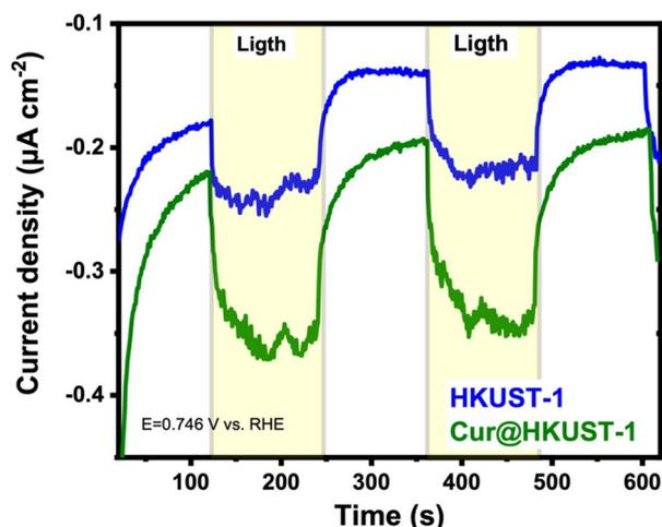
Fig. 5 Chronoamperometry experiments in light/darkness for **HKUST-1** and **Cur@HKUST-1**, evidencing an enhanced photosensitization for the composite.
