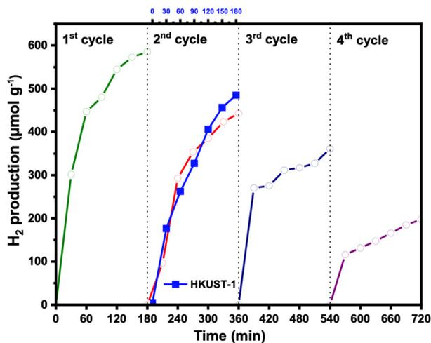
Fig. 11 Photocatalytic hydrogen evolution of **Cur@HKUST-1** after four reaction cycles (1<sup>st</sup> cycle green, 2<sup>nd</sup> cycle red, 3<sup>rd</sup> cycle dark blue, 4<sup>th</sup> cycle purple; **HKUST-1** was just assessed the 1<sup>st</sup> cycle, light blue).
