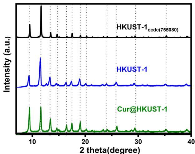
Fig. 2 Diffractograms of **Cur@HKUST-1** (green), **HKUST-1** (blue) synthesized in this work, and the **HKUST-1** monocystal 755080 CCDC reference (black).
