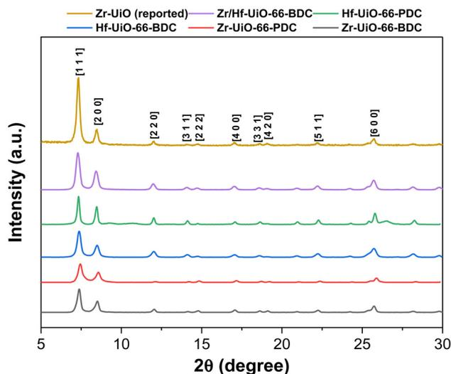
Fig. 1 XRD patterns obtained for UiO-66s.<sup>8,49,50</sup>
