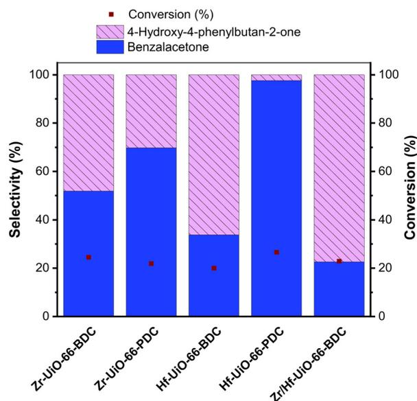
Fig. 6 Selectivity obtained at 20% conversion in UiO-66 catalysts.
