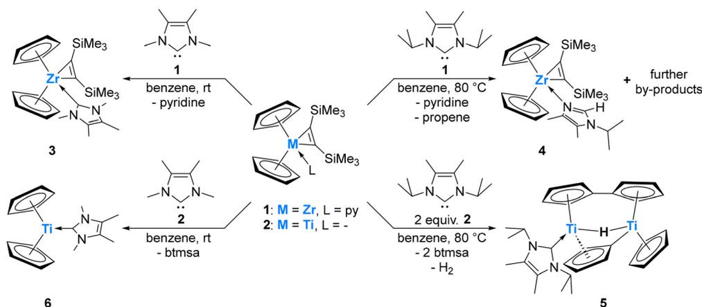
Scheme 2 Reactions of [Cp<sub>2</sub>Ti(btmsa)] (**1**) and [Cp<sub>2</sub>Zr(py)(btmsa)] (**2**) towards IMe<sub>4</sub> and I<sup>1</sup>Pr<sub>2</sub>Me<sub>2</sub> to give complexes **3**, **4**, **5**, and **6**.
