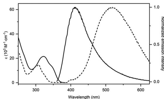
Fig. 2 UV-vis absorption and photoluminescence emission in dilute  $\text{CH}_2\text{Cl}_2$  ( $2 \times 10^{-5} \text{ M}$ ) for the complex  $\text{Si}(\text{O}^1\text{NO}^2)_2$  (solid traces) and the proligand ( $\text{O}^1\text{NO}^2$ ) $\text{H}_2$  (dashed traces). Emission spectra were recorded upon excitation at  $\lambda_{\text{exc}} = 320 \text{ nm}$ .
