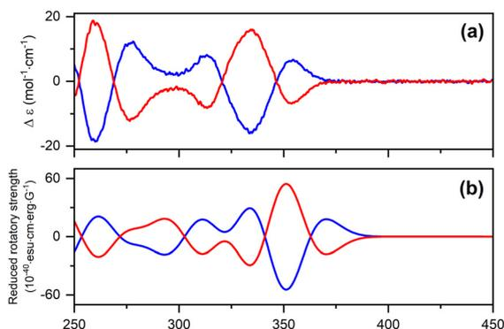
**Fig. 3** (a) Experimental ECD spectra in dilute CH<sub>2</sub>Cl<sub>2</sub> at a concentration of  $2 \times 10^{-4}$  M and (b) computed Boltzmann-weighted ECD spectra for  $\Lambda$ -Si(O<sup>1</sup>NO<sup>2</sup>)<sub>2</sub> (first eluted, blue trace) and  $\Delta$ -Si(O<sup>1</sup>NO<sup>2</sup>)<sub>2</sub> (second eluted, red trace).
