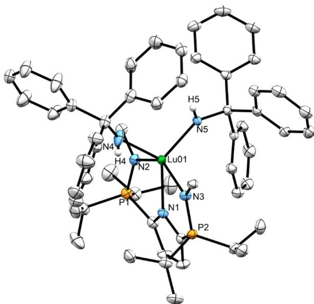
**Fig. 5** Solid-state structure for complex  $8_{\text{CPh}_3}$  with thermal ellipsoids represented at 50% probability. Hydrogen atoms and Pipp groups (except N-C<sub>ipso</sub> carbon atoms) omitted for clarity. Selected bond lengths (Å) and angles (°) for  $8_{\text{CPh}_3}$ : Lu1–N1 2.327(2), Lu1–N2 2.375(2), Lu1–N4 2.153(2), Lu1–N5 2.164(3), P1–N2 1.617(3), N5–Lu1–N4 103.58(9), N3–Lu1–N2 143.59(8), N1–Lu1–N4 132.20(8), N1–Lu1–N5 124.01(9).
