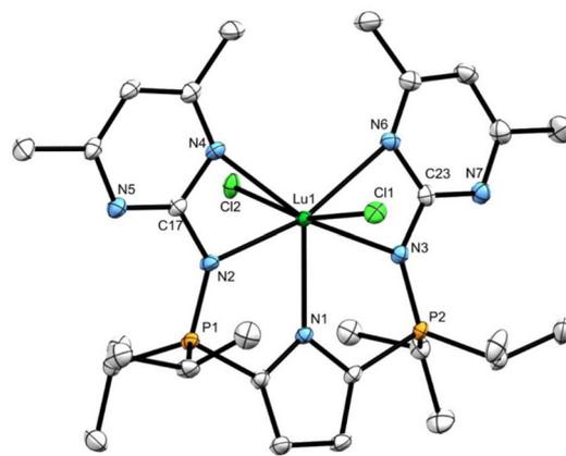
**Fig. 8** Solid-state structure for compound **13** with thermal ellipsoids represented at 50% probability. Hydrogen atoms omitted for clarity. Selected bond lengths (Å) and angles (°) for compound **13**: Lu1–N1: 2.324(2), Lu1–N2: 2.318(2), Lu1–N4: 2.546(2), Lu1–Cl2: 2.5808(8), N2–Lu1–N4: 54.59(6), Cl1–Lu1–Cl2: 162.48(3).
