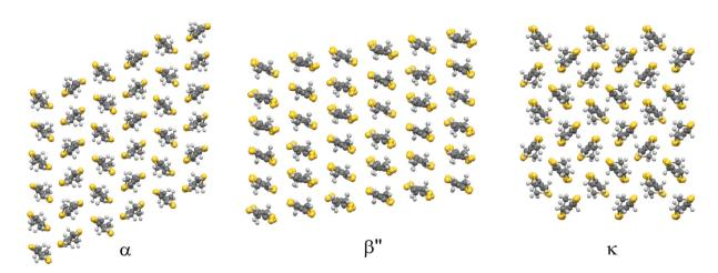
Fig. 2 Alpha, beta", and kappa BEDT-TTF packing arrangements. 10
