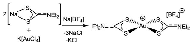
**Scheme 3** Synthesis of  $[\text{Au}(\text{Et}_2\text{dtc})_2][\text{BF}_4]$  (reaction conducted in acetone).
