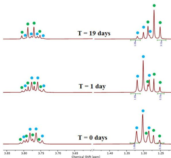
Fig. 10 Comparison of  $^1\text{H}$  NMR spectra (in DMSO- $\text{d}_6$ ) following conversion of the  $[\text{AuCl}_2(\text{Et}_2\text{dtc})]$  mixture, synthesized from water. Blue dots correspond to peaks from the cationic  $[\text{Au}(\text{Et}_2\text{dtc})_2]^+$  species and green dots correspond to peaks from neutral  $[\text{AuCl}_2(\text{Et}_2\text{dtc})]$ .
