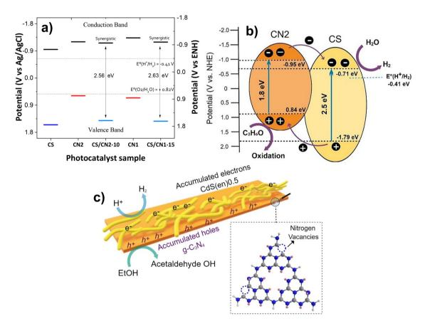
Fig. 12 (a) Band alignments for the materials estimated from the MS plot and band gap energy. (b) Mechanism of the synergistic effect of the CdS/ $g-C_3N_4$  composite under blue-light irradiation. (c) Scheme illustrating the accumulation of electrons in CS nanofibers and holes in CN micro-flakes for  $H_2$  production.
