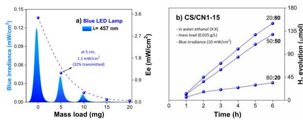
Fig. 6 Plot of blue irradiance measured inside the suspension as a function of the (a) mass load and (b) H2 production profiles of CS/CNX-Y composite suspensions with varying ethanol: water volume ratios.
