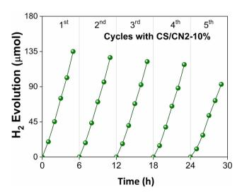
Fig. 8 Profile of  $H_2$  production from ethanol: water solution using the CS/CN2-10 composite over four reaction cycles.
