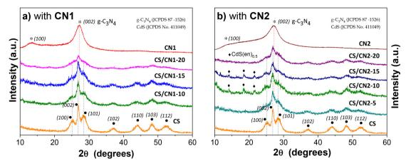
Fig. 1 XRD patterns of heterojunctions of CdS formed on  $g-C_3N_4$  using the solvothermal method: (a) CN1 and (b) CN2 at different contents, along with pure CdS and  $g-C_3N_4$ .
