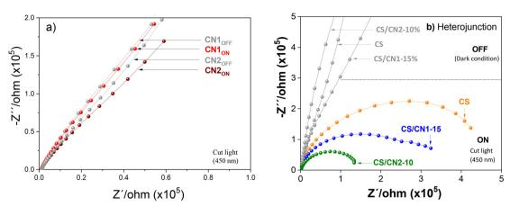
Fig. 11 (a) EIS of the CN1 and CN2 materials, (b) EIS of the CS, CS/CN1-15, and CS/CN2-10 materials under dark and light conditions.
