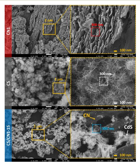
Fig. 4 SEM images of CN1, CS, and heterojunctions of CdS formed on g-C<sub>3</sub>N<sub>4</sub> (CN1) at 15 wt% using the solvothermal method.
