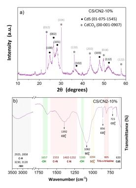
Fig. 9 (a) XRD patterns and (b) FTIR analysis of the used CS/CN2-10 composite after the 4<sup>th</sup> cycle of reaction.
