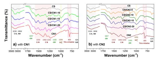
Fig. 2 FTIR analysis of heterojunctions of CdS formed on  $g-C_3N_4$  (a) CN1 and (b) CN2 at different contents using the solvothermal method, along with pure CdS and  $g-C_3N_4$ .
