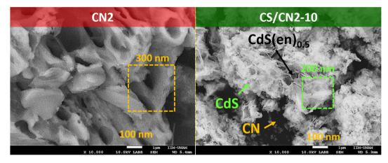
Fig. 5 SEM images of CN2 and heterojunctions of CdS formed on g-C<sub>3</sub>N<sub>4</sub> (CN2) at 10 wt% using the solvothermal method.
