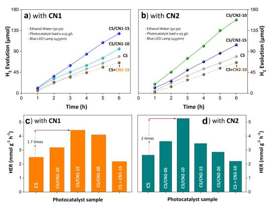
Fig. 7 Profile of  $H_2$  production from ethanol: water solution using 0.025 g  $L^{-1}$  photocatalyst load, prepared (a) with **CN1** samples and (b) with **CN2** samples. (c and d) Profile of standardized  $H_2$  production using composites with **CN1** and **CN2**, respectively.
