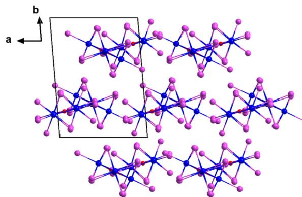
Fig. 8 Section of the crystal structure of  $b\text{-Nb}_4\text{OI}_{11}$ , following the [001] string direction.
