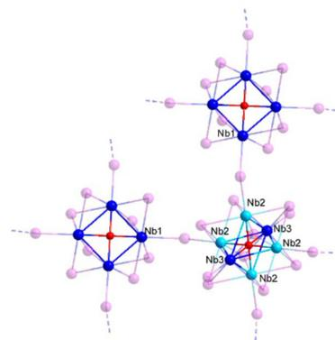
Fig. 5 Cluster connectivity in the structure of  $a\text{-Nb}_4\text{OI}_{11}$  with the equivalent Nb2 positions coloured in cyan. Due to the half-occupation of Nb2 sites, only one pair of Nb2 atoms is present.
