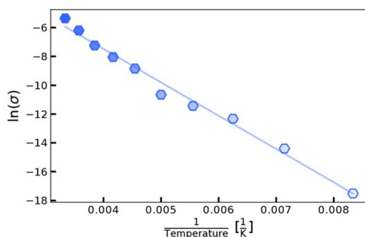
Fig. 10 Arrhenius plot of the electrical conductivity of  $b$ - $\text{Nb}_4\text{OI}_{11}$ , with 20 K temperature steps between 120–300 K. The blue line represents a linear Arrhenius fit to the data.
