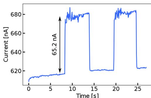
Fig. 11 Photoresponse of  $b$ - $\text{Nb}_4\text{OI}_{11}$  at 300 K toward a 779 nm laser illumination with 1 V bias applied.
