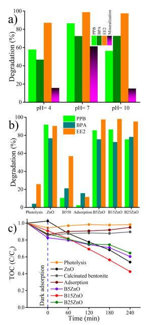
Fig. 5 (a) Effect of pH on the photocatalytic performance of B15ZnO, and (b) degradation and (c) mineralization of the EDC mixture by photolysis, adsorption, and photocatalysis with ZIF-8-derived ZnO, calcined bentonite, and the composite materials (0.5 g  $L^{-1}$  of catalyst, 5 mg  $L^{-1}$  of the PPB, BPA, and EE2 mixture at pH = 7).
