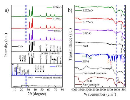
Fig. 1 (a) XRD and (b) FTIR analysis of natural bentonite, calcined bentonite, ZIF-8, ZIF-8-derived ZnO and the composites bentonite-X%/ZnO (X = 5, 15 and 25%).
