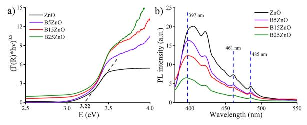
Fig. 4 (a) The Kubelka–Munk function F(R) vs. energy (eV) and (b) photoluminescence spectra of the synthesized materials.
