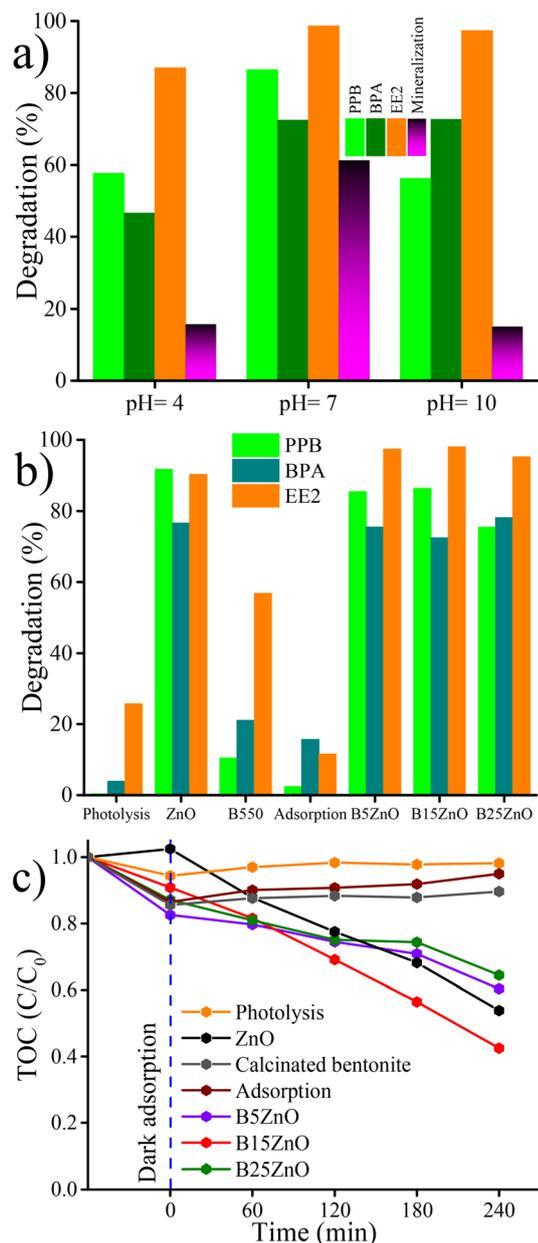
**Fig. 5** (a) Effect of pH on the photocatalytic performance of B15ZnO, and (b) degradation and (c) mineralization of the EDC mixture by photolysis, adsorption, and photocatalysis with ZIF-8-derived ZnO, calcinated bentonite, and the composite materials (0.5 g L<sup>-1</sup> of catalyst, 5 mg L<sup>-1</sup> of the PPB, BPA, and EE2 mixture at pH = 7).
