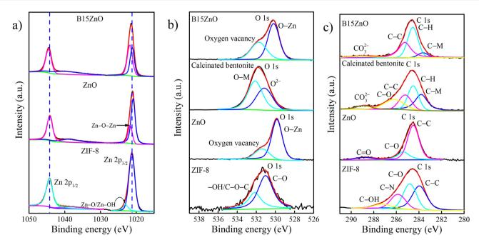
Fig. 3 High-resolution XPS spectra of (a) Zn 2p for ZIF-8, ZIF-8-derived ZnO, and B15ZnO, and (b) O 1s and (c) C 1s for ZIF-8, ZIF-8-derived ZnO, calcined bentonite and B15ZnO.
