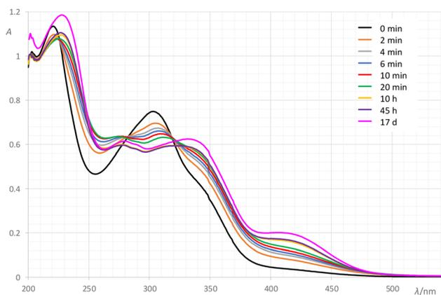
Fig. 3 Time-dependent UV-Vis spectra of a reaction mixture of NH<sub>4</sub>VO<sub>3</sub> and H<sub>2</sub>VIH in methanol at room temperature.
