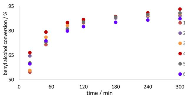
**Fig. 6** Kinetic profiles of benzyl alcohol conversion with V catalysts. The reaction temperature was 80 °C and TBHP in decane was used as the oxidizing agent. Reaction conditions: time, 5 h; temperature, 80 °C,  $n(\text{catalyst})/n(\text{cyclooctene})/n(\text{oxidant}) = 0.1 \text{ mmol}/20 \text{ mmol}/40 \text{ mmol}$ .
