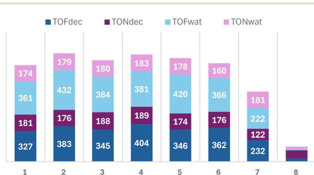
**Fig. 7** Comparison of TOF<sub>20 min</sub> and TON values for V catalysts 1–6 and Mo catalysts 7 and 8, with TBHP in decane and water as the oxidizing agent, for benzyl alcohol oxidation.
