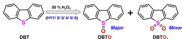
**Scheme 2** Catalytic oxidation of DBT by using **HY1/2/3/4/5/6** as the catalyst.
