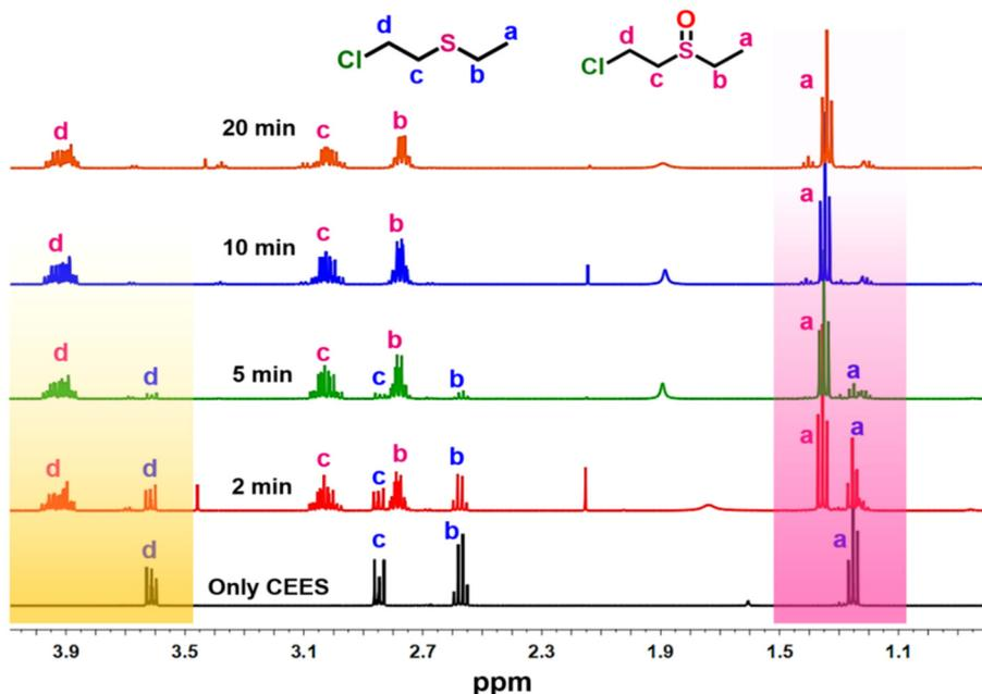
**Fig. 9** Selected region of stacked <sup>1</sup>H NMR spectra of CEES, after 2, 5, 10 and 20 min of the reaction product by using CDCl<sub>3</sub> as a solvent.
