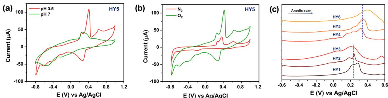
Fig. 7 Cyclic voltammograms (CVs) of (a) HY5 in pH 3.5 and 7; (b) HY5 in  $N_2$  or  $O_2$ . Differential pulse voltammograms (DPVs) of HY1–HY6 (c) anodic scan in 0.1 M  $Na_2SO_4$  at pH 3.5. All the CVs were recorded at the scan rate of  $50 \text{ mV s}^{-1}$ .
