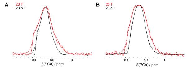
Fig. 4  $^{71}$ Ga solid state MAS NMR spin-echo spectra recorded at 259 MHz (red) or 306 MHz (black) (A) [Ga(Br<sub>2</sub>-HQ)<sub>3</sub>], and (B) [Ga (HQ)<sub>3</sub>]·0.5CH<sub>3</sub>CO<sub>2</sub>H. The peaks were fitted as single sites (red dashed and black dashed lines). Spectra are scaled to equal maxima. The narrowing of peaks at higher frequency is evident.
