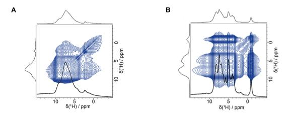
Fig. 6 <sup>1</sup>H-<sup>1</sup>H NOESY solid state MAS spectra at 850 MHz of (A) [Ga(Br<sub>2</sub>-HQ)<sub>3</sub>] and (B) [Ga(HQ)<sub>3</sub>]·0.5 CH<sub>3</sub>CO<sub>2</sub>H (mixing time of 220 ms).
