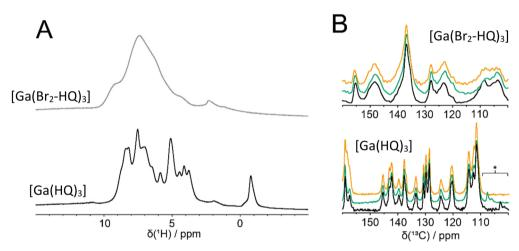
Fig. 5 (A)  $^{1}$ H NMR solid-state NMR spectra of  $[Ga(Br_{2}-HQ)_{3}]$  and  $[Ga(HQ)_{3}]\cdot 0.5CH_{3}CO_{2}H$  recorded at 23.5 T (1 GHz). (B) 20 T (214 MHz)  $^{13}$ C solid state CPMAS NMR spectra of  $[Ga(Br_{2}-HQ)_{3}]$  (top) and  $[Ga(HQ)_{3}]\cdot 0.5$  CH $_{3}CO_{2}H$  (bottom) at spinning rates of 10 kHz (black), 11 kHz (blue) and 12 kHz (orange). Peaks assigned to the complexes have chemical shifts independent of spinning rate. \* = Spinning side bands.
