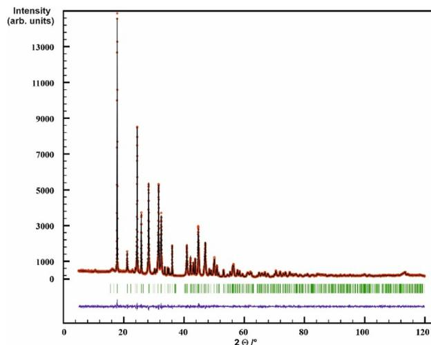
Fig. 4 Rietveld refinement of the XRD powder pattern of  $\text{La}_2(\text{CN}_2)_3$ . Observed intensities are marked as red circles, and calculated intensities as black lines. Bragg positions are marked as green lines, the difference curve  $I_{\text{observed}} - I_{\text{calculated}}$  as blue line.
