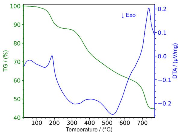
Fig. 1 Thermogravimetric analysis (TGA) combined with differential thermal analysis (DTA) of La(HC<sub>3</sub>N<sub>3</sub>O<sub>3</sub>)(H<sub>2</sub>C<sub>3</sub>N<sub>3</sub>O<sub>3</sub>)(H<sub>2</sub>O)<sub>3</sub>.
