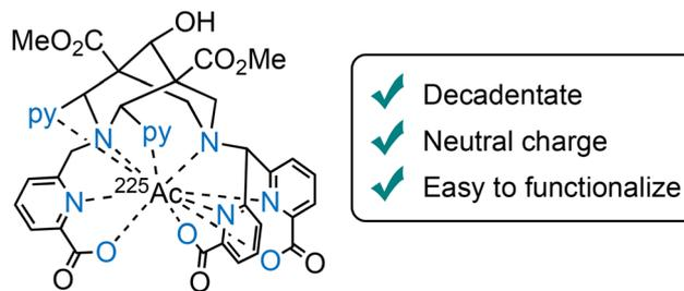
Fig. 8 Ac-225 complex of the decadentate bispidine chelator  $L^{24}$  for the selective coordination of Ac<sup>III</sup>.
