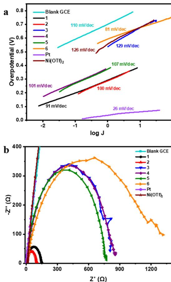
Fig. 3 (a) Tafel slope and (b) Nyquist plot of 1–6 in comparison to GCE, Pt, and Ni(OTf)<sub>2</sub> standards (after peak reductive cycling in 0.5 M aq. H<sub>2</sub>SO<sub>4</sub>).
