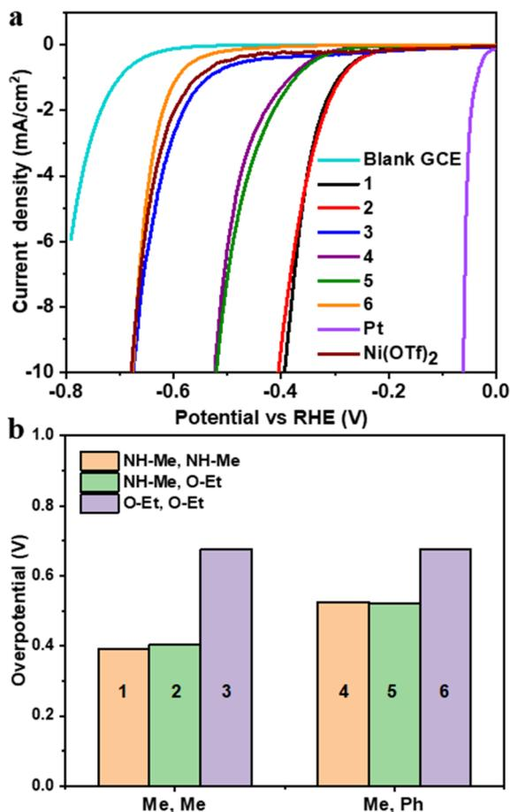
Fig. 2 (a) LSV of electrodes 1–6 compared to GCE, Pt, and Ni(OTf)<sub>2</sub> standards after peak reductive cycling (400 cy, 400 cy, 900 cy, 100 cy, 700 cy and 100 cy for 1–6, respectively) in 0.5 M aq. H<sub>2</sub>SO<sub>4</sub> and (b) graphical representation of the overpotential (at current density of  $-10 \text{ mA cm}^{-2}$ ) trend for 1–6 with changes in the pendent group (NH-Me or O-Et) and ligand backbone (Me, Me or Me, Ph).
