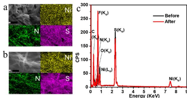
**Fig. 5** Elemental mapping of 2 (a) as drop cast on GCE, showing SEM image (grayscale), nickel (yellow), nitrogen (green) and sulfur (pink) and (b) after 1000 reductive cycles. Scale bars at the bottom of SEM image correspond to 10 μm. (c) Comparative elemental plot before and after 1000 reductive cycle.
