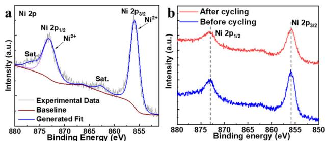
Fig. 6 XPS data for 2 showing (a) the fitted  $Ni^{2+}$  data before reductive cycling and (b) the Ni region before and after 1000 reductive cycles.
