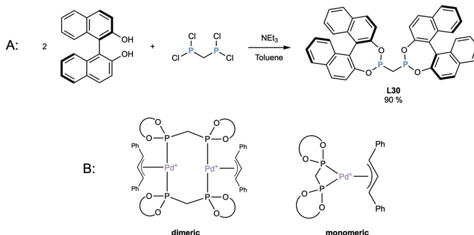
Fig. 8 (A) Synthesis of ligand **L30**. (B) Pd species observed in solution. PF<sub>6</sub><sup>-</sup> counteranions have been omitted for clarity.
