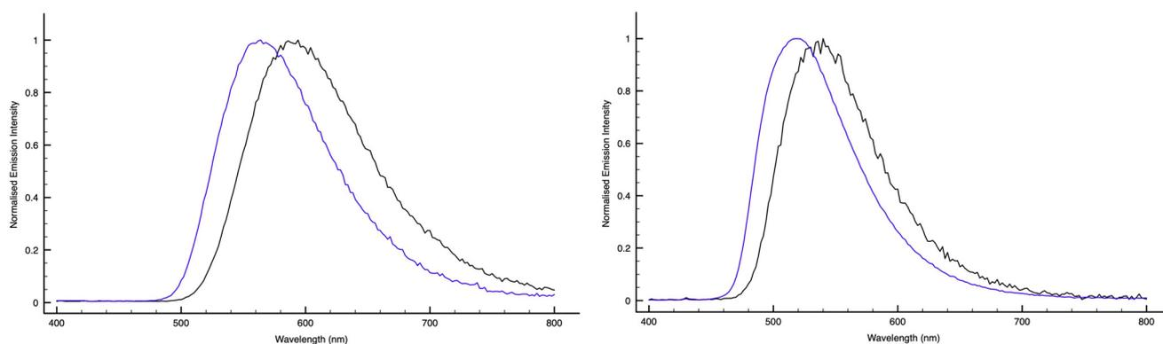
Fig. 4 (left) Normalized emission profiles of  $[\text{Ir}(\text{ppyCN})_2(\text{PTZ})]$  (black line) and  $[\text{Ir}(\text{ppyCN})_2(\text{PTZ}-\text{Me})]^+$  (blue line); (right)  $[\text{Ir}(\text{F}_2\text{ppy-CN})_2(\text{PTZ})]$  (black line) and  $[\text{Ir}(\text{F}_2\text{ppy-CN})_2(\text{PTZ}-\text{Me})]^+$  (blue line).
