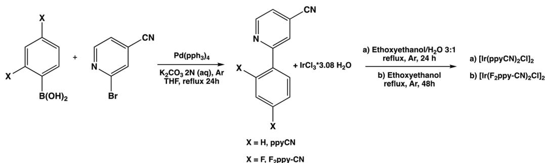
**Scheme 1** Synthesis of  $[\text{Ir}(\text{ppyCN})_2\text{Cl}]_2$  and  $[\text{Ir}(\text{F}_2\text{ppy-CN})_2\text{Cl}]_2$ .
