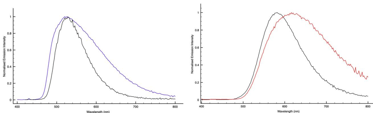
Fig. 5 (left) Normalized emission profiles of  $[\text{Ir}(\text{F}_2\text{ppy-CN})_2(\text{PYZ})]$  (black line) and  $[\text{Ir}(\text{F}_2\text{ppy-CN})_2(\text{PYZ}-\text{Me})]^+$  (blue line); (right)  $[\text{Ir}(\text{ppyCN})_2(\text{PYZ})]$  (black line) and  $[\text{Ir}(\text{ppyCN})_2(\text{PYZ}-\text{Me})]^+$  (red line).
