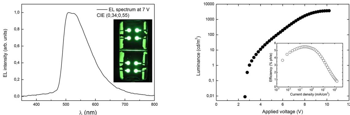
**Fig. 9** (left) Electroluminescence spectra at 7 V of the OLED. In the inset is reported a photo of a green OLED; (right) luminance vs. applied voltage and external efficiency vs. current density (inset) of the OLED.
