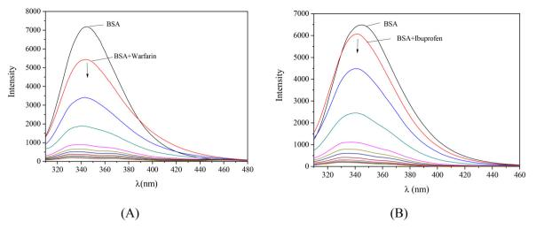
Fig. 8 Fluorescence emission spectra ( $\lambda_{\text{excitation}}$  = 295 nm) of a buffer solution (150 mM NaCl and 15 mM trisodium citrate at pH 7.0) of BSA (3  $\mu$ M) in the presence of (A) warfarin (3 μM) or (B) ibuprofen (3 μM), upon addition of increasing amounts of complex 2. The arrows show the changes of intensity upon increasing amounts of the complexes.
