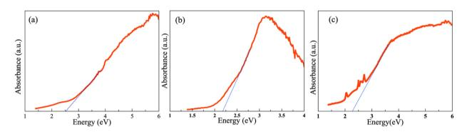
$\textbf{Fig. 7} \quad \text{Optical absorption plot of polycrystalline (a) } \\ \text{La}_{3}\text{Si}_{2}\text{Se}_{1.21}\text{S}_{6.79}\text{I}, \text{ (b) } \\ \text{Ce}_{3}\text{Si}_{2}\text{Se}_{1.39}\text{Se}_{6.61}\text{I}, \text{ and (c) } \\ \text{Pr}_{3}\text{Si}_{2}\text{Se}_{1.22}\text{Se}_{6.78}\text{I}. \\ \text{Secondary of the properties of the propert$
