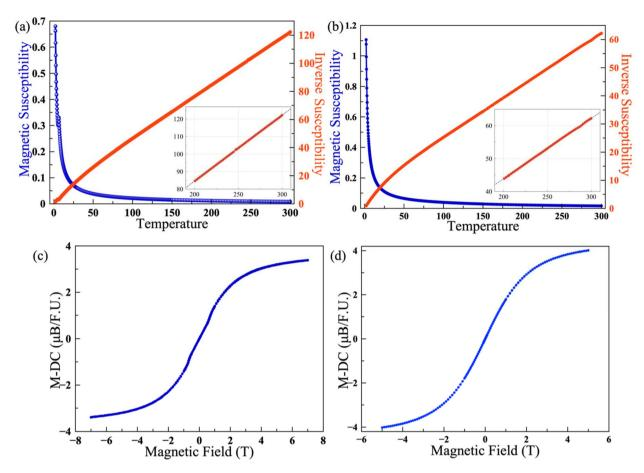
Fig. 6 Molar susceptibility and inverse molar susceptibility vs. temperature plots for polycrystalline (a)  $Ce_3Si_2Se_{1.39}S_{6.61}$  and (b)  $Nd_3Si_2Se_{1.18}S_{6.82}$  measured in an applied field of 1000 Oe; magnetization as a function of applied field plots for polycrystalline (c)  $Ce_3Si_2Se_{1.39}S_{6.61}$  and (d)  $Nd_3Si_2Se_{1.18}S_{6.82}$ I measured at 2 K.
