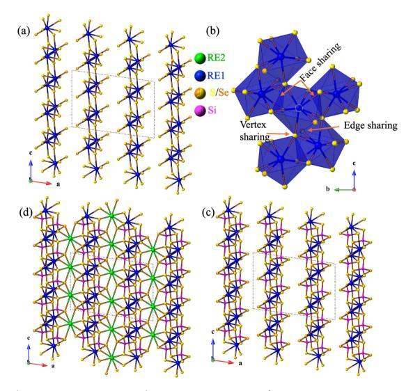
Fig. 4 (a)  $2D_{\infty}^{1}[RE1Q_{5}]$  layers along the b-axis, (b)  $2D_{\infty}^{1}[RE1Q_{5}]$  ribbons along the a-axis, (c)  $\frac{2}{\infty}[RE1SiQ_{4}]$  layers viewed along the b-direction, and (d) total 3D view of  $\frac{3}{\infty}[RE_{3}Si_{2}Se_{x}S_{8-x}]^{1+}$ , with RE2Q<sub>8</sub> bicapped trigonal prisms bridging between  $\frac{2}{\infty}[RE1SiQ_{4}]^{1-}$  layers.
