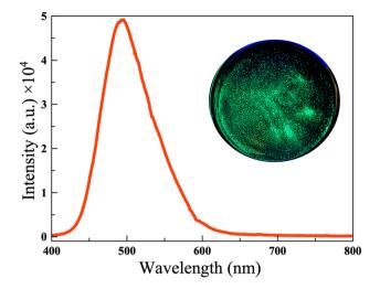
Fig. 8 Emission spectra of the Ce<sub>3</sub>Si<sub>2</sub>Se<sub>1.39</sub>S<sub>6.61</sub>I single crystal (the inset figure shows the green color of the sample under exposure to UV light).
