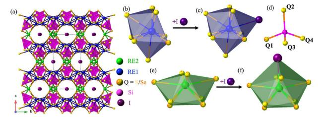
Fig. 3 The (a) unit cell view of  $RE_3Si_2Se_xS_{8-x}I$  compounds, (b)  $RE1Q_8$  bicapped trigonal prism, (c)  $RE2Q_8$  bicapped trigonal prism, (d)  $SiQ_4$  tetrahedron, (e)  $RE2Q_8$  bicapped trigonal prism, and (f)  $RE1Q_8I$  tricapped trigonal prism.
