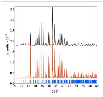
Fig. 2 The PXRD pattern of the polycrystalline  $Nd_3Si_2Se_{1.18}S_{6.82}l$  compound (simulated pattern (red), experimental pattern (black) and Bragg position (blue)).
