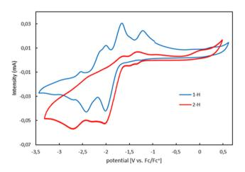
Fig. 5 [-3.5 V; -0.7 V] region of cyclic voltammogram of 3.0 mM THF solutions of complex 1-H (blue) and 2-H (red) recorded in 0.1 M  $[\mathrm{NBu_4}][\mathrm{PF_6}]$  under  $\mathrm{N_2}$  at 25 °C, at a scan rate of 100 mV s $^{-1}$ , referenced against Fc+/Fc.
