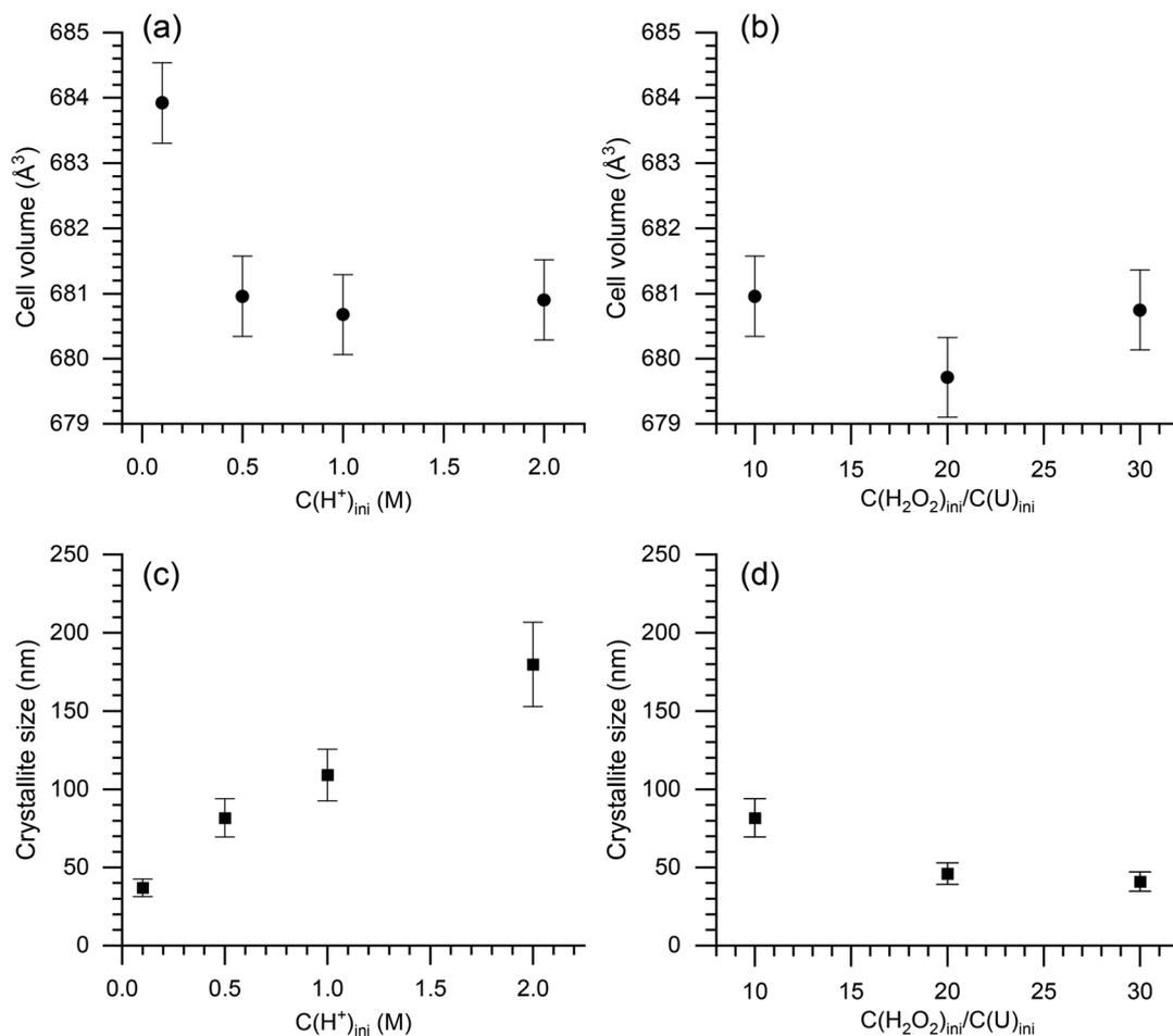
Fig. 5 Unit cell volume of uranium(vi) peroxide for different initial  $H^+$  concentrations (a) and for different initial  $C(H_2O_2)_{ini}/C(U)_{ini}$  molar ratios (b); crystallite size of uranium(vi) peroxide for different initial  $H^+$  concentrations (c) and for different initial  $C(H_2O_2)_{ini}/C(U)_{ini}$  molar ratios (d).
