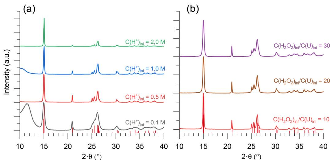
Fig. 4 PXRD patterns of studtite precipitates obtained for various  $H^+$  concentrations (0.1 M in black, 0.5 M in red, 1.0 M in blue, and 2.0 M in green), with  $C(H_2O_2)_{ini}/C(U)_{ini} = 10$  and  $C(U)_{ini} = 0.07$  M (a) and for different initial  $C(H_2O_2)_{ini}/C(U)_{ini}$  molar ratios (10 in red, 20 in brown and 30 in purple) with  $C(H^+)_{ini} = 0.5$  M and  $C(U)_{ini} = 0.07$  M (b); PXRD lines in red correspond to uranium(vi) peroxide from Burns *et al.*<sup>58</sup>
