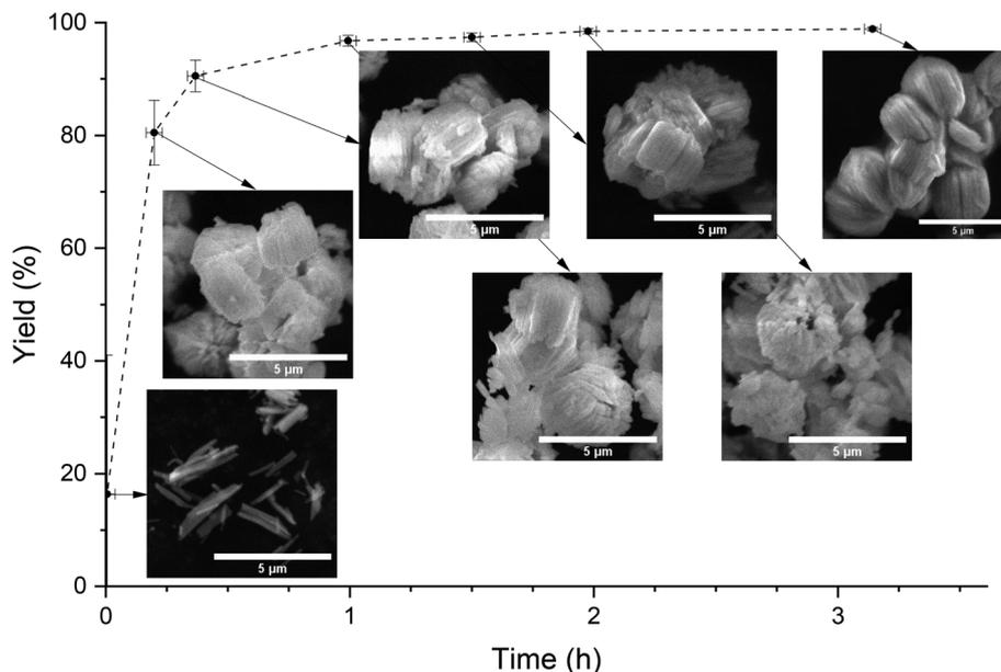
Fig. 3 SEM micrographs of uranium(vi) peroxide obtained during precipitation for  $C(H^+)_{ini} = 0.5$  M,  $C(H_2O_2)_{ini}/C(U)_{ini} = 20$  and  $C(U)_{ini} = 0.07$  M. The dashed line is a guide to the eye and does not represent any mathematical fit.
