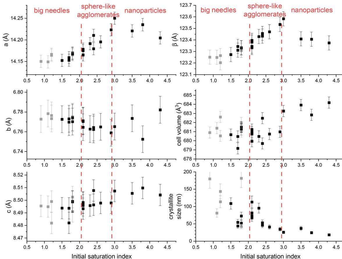
**Fig. 6** Lattice parameters ( $a$ ,  $b$ ,  $c$  and  $\beta$ ), unit cell volume and crystallite size of studtite crystals as a function of initial saturation index. Grey points are  $U(VI)$  peroxide samples from precipitation that have not reached equilibrium. Refinement results are available in Table ESI 2.†
