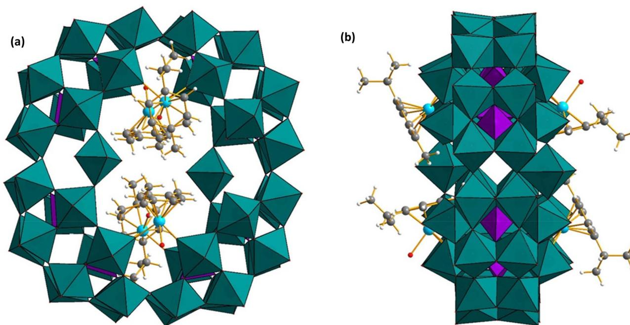
**Fig. 16** Combined polyhedral/ball-and-stick representation of  $[\{K(H_2O)\}_3\{Ru(p\text{-cymene})(H_2O)\}_4P_8W_{49}O_{186}(H_2O)_2\}]^{27-}$ . (a) Front-view, (b) side-view. Color code:  $WO_6$  octahedra (green),  $PO_4$  tetrahedra (pink), Ru (sky blue), O (red), C (grey), H (white).<sup>127</sup>
