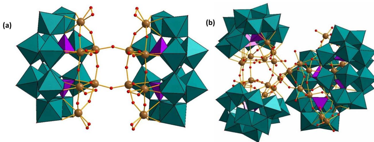
**Fig. 5** Combined polyhedral, ball-and-stick representations of (a)  $[H_{13}\{Nb_6(O_2)_4P_2W_{12}O_{57}\}_2]^{7-}$  and (b)  $[H_{14}\{P_2W_{12}Nb_7O_{63}(H_2O)_2\}_4\{Nb_4O_4(OH)_6\}]^{16-}$ , respectively. Color code:  $WO_6$  octahedra (green),  $PO_4$  tetrahedra (pink), Nb (brown), O (red).<sup>67</sup>
