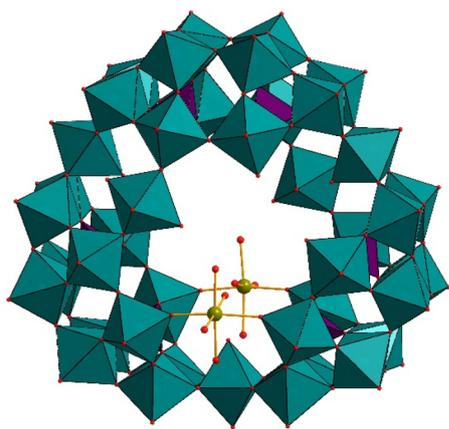
Fig. 6 Combined polyhedral/ball-and-stick representation of  $[K_3C\{Mn(H_2O)_4\}_2\{WO_2(H_2O)_2\}_2\{WO(H_2O)\}_3\{P_2W_{12}O_{48}\}_3]^{19-}$ . Color code:  $WO_6$  octahedra (green),  $PO_4$  tetrahedra (pink), Mn (teal), O (red).<sup>71</sup>
