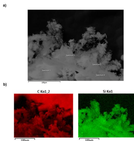
Fig. 8 (a) SEM backscattered-electron image for the dark-grey precipitate obtained from the photolysis of silaspiro-[4.4]-2,3,7,8-tetramethyl-2,7-nonadiene (**SpiroSi**); SEM data was collected at  $15\text{ keV}$ ; (b) EDX elemental maps for the dark-grey precipitate obtained from the photolysis of silaspiro-[4.4]-2,3,7,8-tetramethyl-2,7-nonadiene (**SpiroSi**) in THF.
