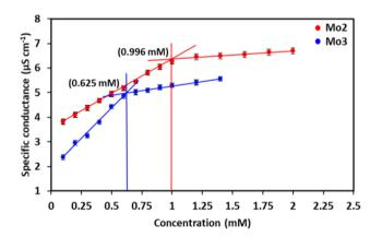
Fig. 3 Determination of critical micelle concentration (CMC) of Mo2 and Mo3.
