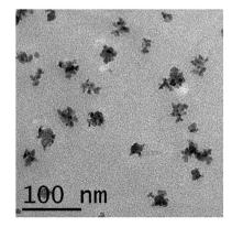
Fig. 4 HR-TEM image of metallomicellar complex Mo3.
