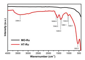
Fig. 2 FTIR spectra of MO-Ru and HT-Ru.
