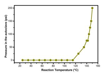
Fig. 12 Measurement of the pressure inside the autoclave during the temperature increase in the hydrogenation of LA with FA catalyzed by MO-Ru.
