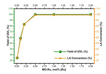
Fig. 9 Influence of the catalyst amount (MO-Ru) on the hydrogenation of LA with FA. Reaction conditions: MO-Ru (based on Ru content), LA (9.8 mmol), formic acid (19.6 mmol),  $H_2O$  (4 mL), 150 °C, 1.5 h.
