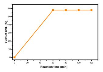
Fig. 11 Test of heterogeneity of the catalyst MO-Ru.
