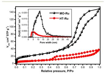
Fig. 3 Nitrogen isotherm at -196 °C and PSD for MO-Ru and HT-Ru.
