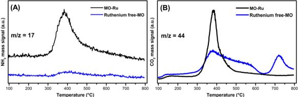
Fig. 6 (A) NH<sub>3</sub>-TPD profiles for MO-Ru and ruthenium-free MO (Mg/Al) and (B) CO<sub>2</sub>-TPD profiles for MO-Ru and ruthenium-free MO (Mg/Al).
