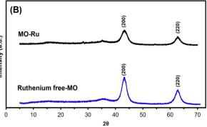
Fig. 1 (A) XRD pattern of HT-Ru and ruthenium-free HT (Mg/Al) and (B) XRD pattern of MO-Ru and ruthenium-free MO (Mg/AL).
