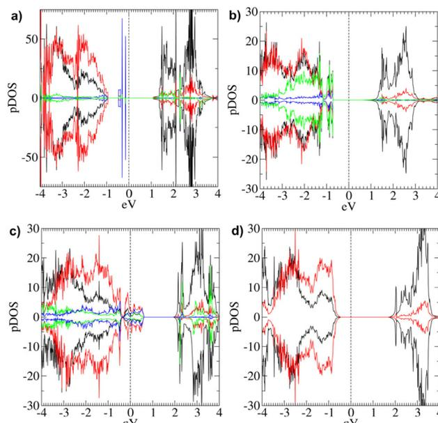
**Fig. 9** pDOS computed for models (a)  $[\text{Ni}_{64}\text{O}_{64}]\text{2H-2(OH)}$ ; (b)  $[\text{Ni}_{24}\text{O}_{24}]\text{4H}$ ; (c)  $[\text{Ni}_{24}\text{O}_{24}]\text{4(OH)}$ ; (d)  $[\text{Ni}_{24}\text{O}_{24}]\text{2H-2(OH)}$ . The vertical dashed line represents the Fermi level position. Positive curves: spin-up components; negative curves: spin down components; black lines: Ni d-states; red lines: O 2p-states; green lines: Ni\* d-states; blue lines: hydroxyl O 2p-states.
