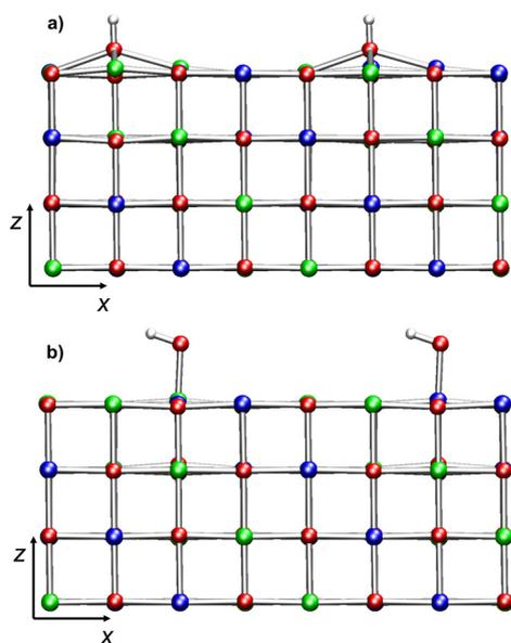
**Fig. 4** Ball-and-stick representation (projected on the  $xz$  plane) of dihydroxylated NiO(100) model slabs mimicking a low concentration of surface hydroxyl groups. (a)  $[\text{Ni}_{64}\text{O}_{64}]2\text{H}$ , containing two H, each bonded to an O atom of the top layer; (b)  $[\text{Ni}_{64}\text{O}_{64}]2(\text{OH})$ , containing two neutral –OH defects bonded to Ni atoms with opposite spin. Color codes: red, O; blue, Ni (spin-up); green, Ni (spin-down); white, H.
