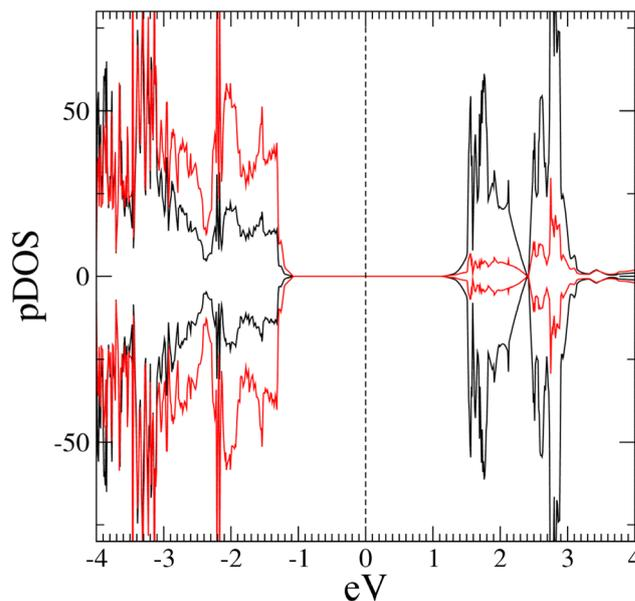
**Fig. 3** pDOS calculated for RegSurf 2 ( $\text{Ni}_{64}\text{O}_{64}$ ). The vertical dashed line represents the position of the Fermi level, conventionally set to 0. Positive curves: spin-up components; negative curves: spin-down components. Black and red lines refer to Ni d-states and O 2p-states, respectively.
