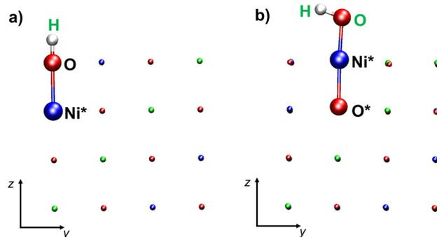
**Scheme 1** Schematic representations of: (a) an –OH defect formed by binding an H atom to a top-layer oxygen; (b) an –OH defect formed by binding a hydroxyl group to a top layer Ni atom. Atoms directly involved in the defect are highlighted as spheres. Color codes: red, O; blue, Ni (spin-up); green, Ni (spin-down). The (a) H and (b) OH atoms adsorbed on the NiO(100) surface are labeled in green; Ni\*: Ni atom bearing the –OH group; O\*: O atom bonded to Ni\*.
