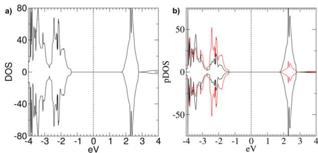
**Fig. 2** (a) DOS and (b) pDOS calculated for Bulk 1 ( $\text{Ni}_{32}\text{O}_{32}$ ). The vertical dashed line represents the position of the Fermi level, conventionally set to 0. Positive curves: spin-up components; negative curves: spin-down components. Black and red lines in (b) refer to Ni d-states and O 2p-states.
