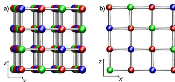
Fig. 1 Ball-and-stick representations of (a) bulk NiO and (b) NiO(100) projected on the xz plane. (a) Model Bulk 1 (Ni<sub>32</sub>O<sub>32</sub>); (b) model RegSurf 1 (Ni<sub>32</sub>O<sub>32</sub>). Color codes: red, O; blue, Ni (spin-up); green, Ni (spin-down).
