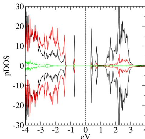
**Fig. 7** pDOS computed for the slab model  $[\text{Ni}_{24}\text{O}_{24}]2\text{H}$ . The vertical line represents the Fermi level position. Positive curves: spin-up components; negative curves: spin down components; black lines: Ni d-states; red lines: oxygen 2p-states; green lines: hydroxyl O 2p-states.
