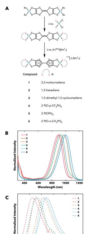
Fig. 1 (A) Synthesis of new Pt-capped TTFtt analogs. See ESI $\dagger$  for further details and procedures. BAr<sup>F</sup><sub>4</sub> $^-$  = tetrakis[3,5-bis(trifluoromethyl) phenyl]borate. (B) Absorption of new analogs in dichloromethane (DCM) at 298 K. (C) Photoluminescence (PL) of new analogs in CH<sub>2</sub>Cl<sub>2</sub> (2, 4) and CD<sub>2</sub>Cl<sub>2</sub> (1, 3, 5, 6) at 298 K.
