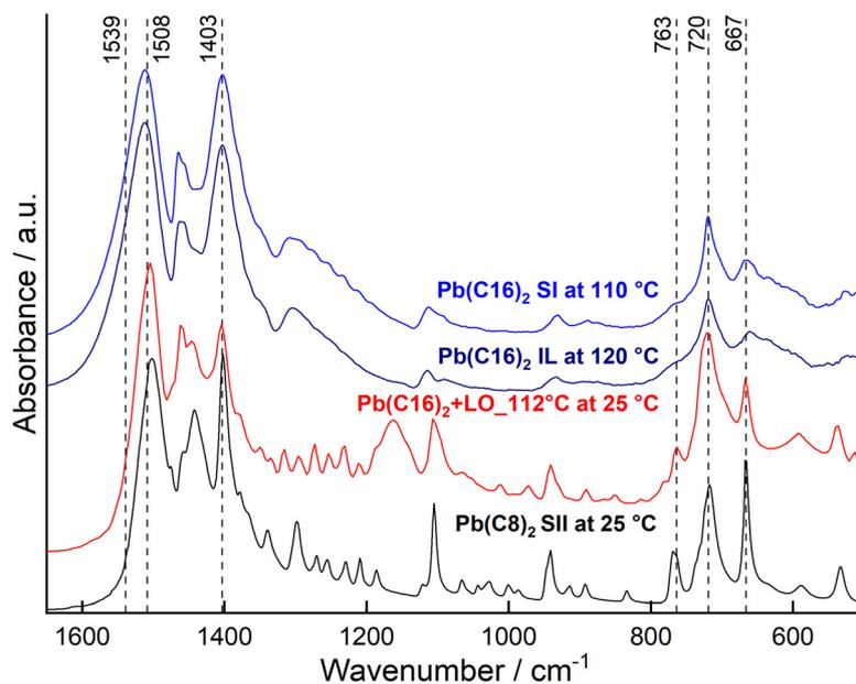
**Fig. 7** Comparison of  $\text{Pb}(\text{C8})_2$  SII phase,  $\text{Pb}(\text{C16})_2$  SI and IL phases and  $\text{Pb}(\text{C16})_2 + \text{LO}_{112\text{ }^\circ\text{C}}$ . The spectra of powder  $\text{Pb}(\text{C16})_2$  cooling from  $150$  to  $35\text{ }^\circ\text{C}$  are present in Fig. S10, ESI.†
