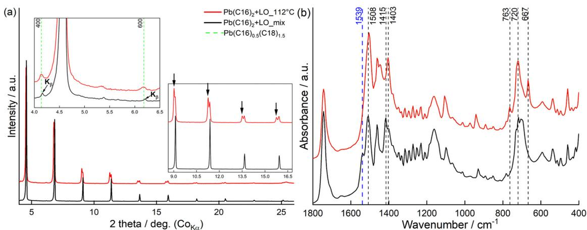
**Fig. 5** Comparison of XRPD (a) and FTIR (b) before ( $\text{Pb}(\text{C16})_2 + \text{LO\_mix}$ , black line) and after ( $\text{Pb}(\text{C16})_2 + \text{LO}_{112\text{ °C}}$ , red line) the treatment. XRPD patterns (a) are normalized to specify intensity increase of mixed lead palmitate stearate signals (lines 400 and 600) compared to the  $K_{\beta}$  lines.
