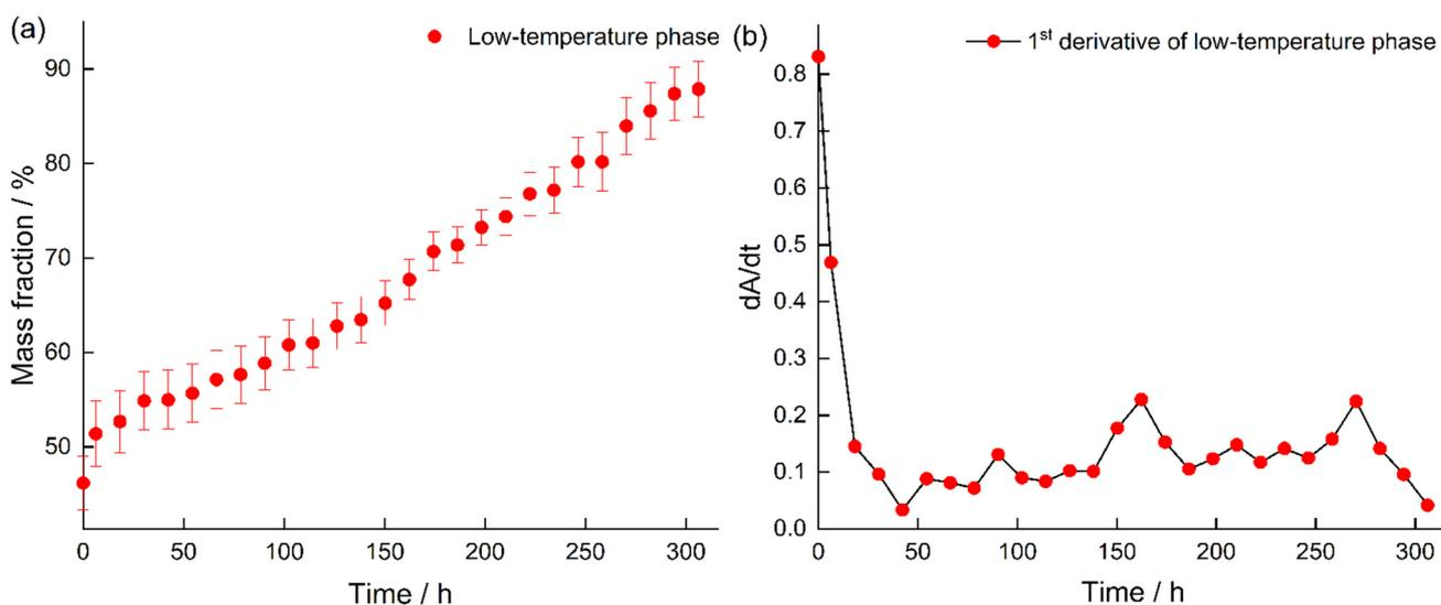
Fig. 10 Concentration–time profile of low-temperature  $\text{Pb}(\text{C16})_2$  phase in the sample  $\text{Pb}(\text{C16})_2 + \text{LO}_{112} \text{ } ^\circ\text{C}$  (a) and its first derivative (b).
