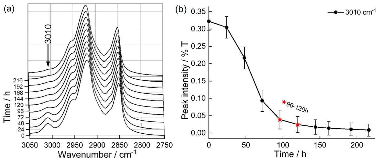
Fig. 11 FTIR spectra of the sample  $\text{Pb}(\text{C16})_2 + \text{LO}_{112} \text{ } ^\circ\text{C}$  normalized to the prominent methylene asymmetric stretching band at  $2922 \text{ cm}^{-1}$  (a) and intensity change over time of deconvoluted band at  $3010 \text{ cm}^{-1}$  (b). Deconvolution example is present in ESI (Fig. S17†).
