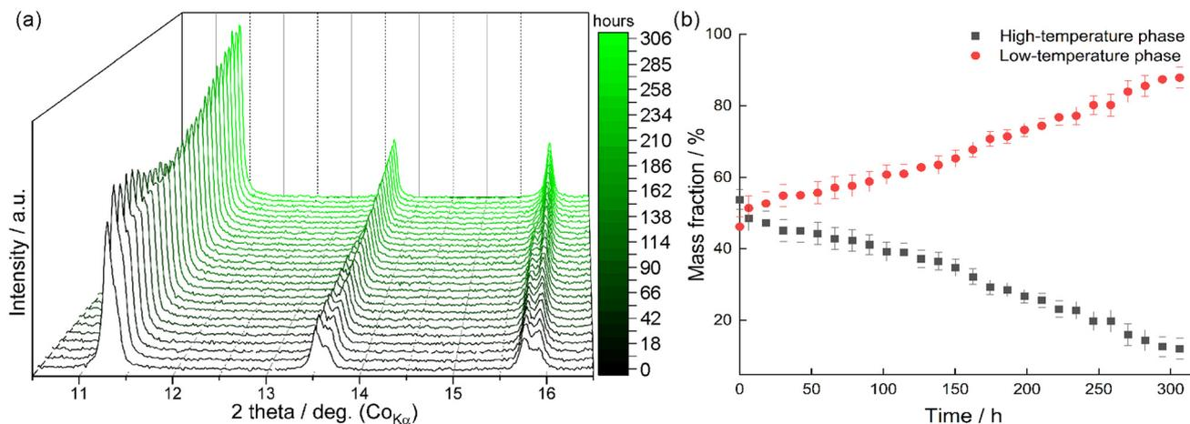
Fig. 9 Progress of transformation in the sample  $\text{Pb}(\text{C16})_2 + \text{LO}_{112} \text{ } ^\circ\text{C}$  followed by XRPD (a) and concentration profiles of both phases (b). Details of fitting are present in Fig. S15 and Table S4, ESI†
