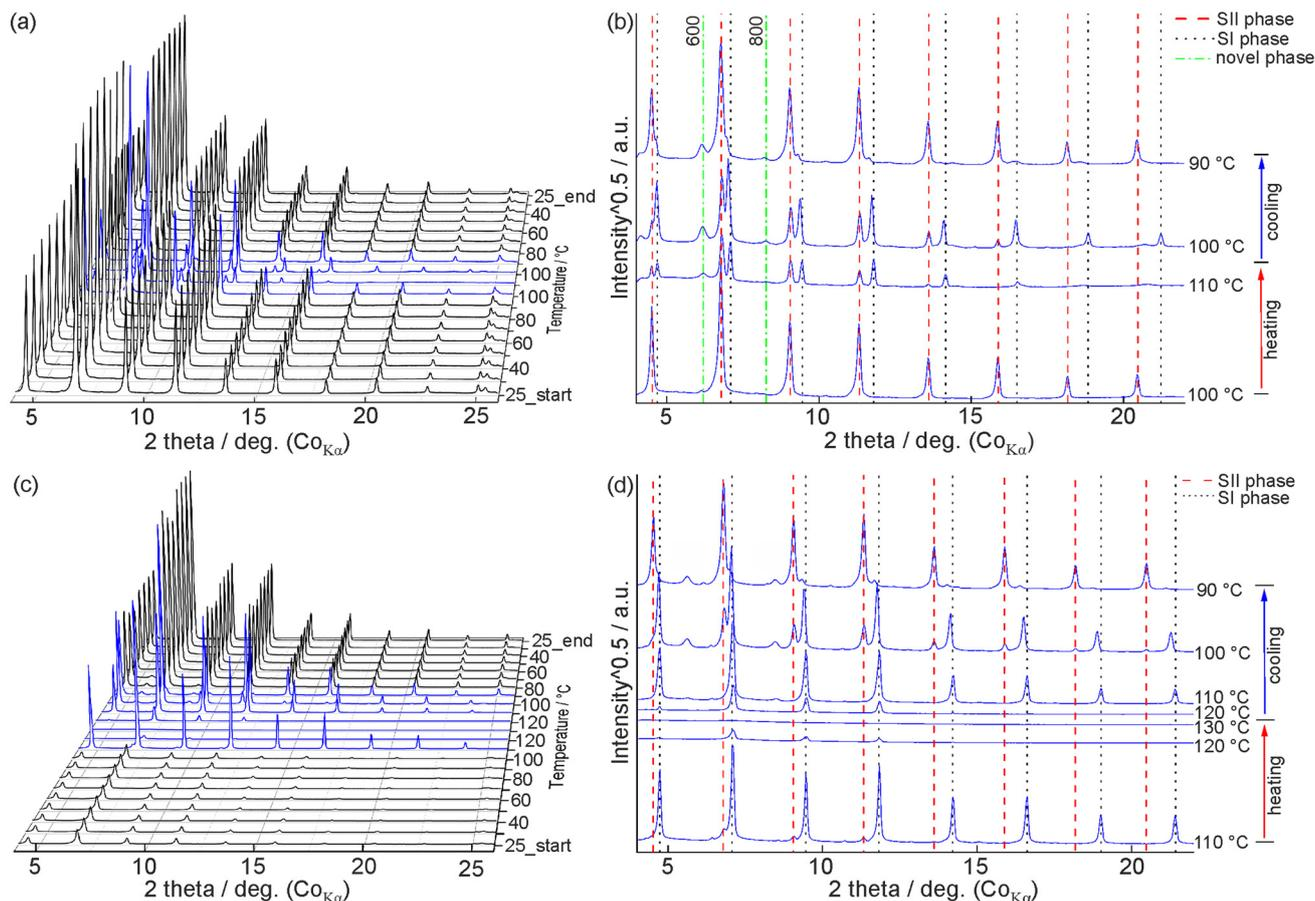
**Fig. 2** *In situ* HT-XRPD patterns of Pb(C16)<sub>2</sub> + LO<sub>mix</sub> (a and b) and powder Pb(C16)<sub>2</sub> (c and d). Measurement progression during heating/cooling cycles (a and c) and selected patterns at particular temperatures (b and d). The patterns were collected from 30 °C onwards with an increment of 10 °C (a and c).
