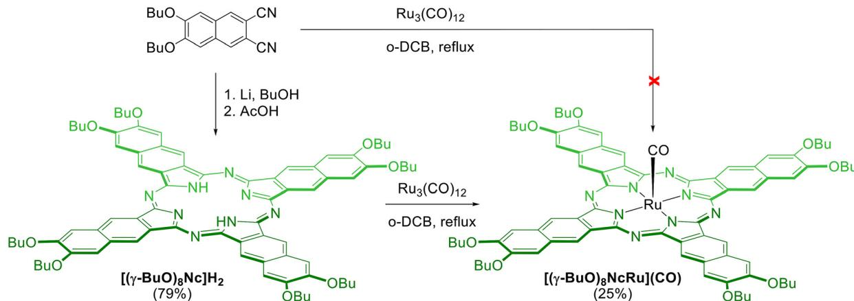
Scheme 1 Synthesis of the ruthenium naphthalocyanine  $[(\gamma\text{-BuO})_8\text{NcRu}](\text{CO})$ .
