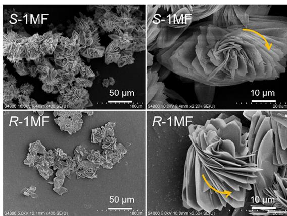
Fig. 2 SEM images of the self-assembled products of  $\text{In}(\text{NO}_3)_3$ / $S$ -,  $R$ -pempH<sub>2</sub> in 90 vol% IPA/H<sub>2</sub>O at 100 °C (**S-1MF** and **R-1MF**).
