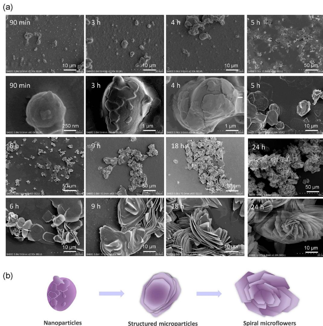
**Fig. 4** (a) SEM images of the self-assembled products of  $\text{In}(\text{NO}_3)_3/\text{S-pempH}_2$  in 90 vol% IPA/ $\text{H}_2\text{O}$  at 100 °C for different reaction times. (b) Proposed mechanism for the formation of spiral microflowers.
