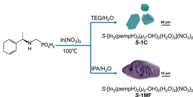
**Scheme 1** Synthetic routes to **S**-1C and **S**-1MF in mixtures of TEG/H<sub>2</sub>O and IPA/H<sub>2</sub>O.
