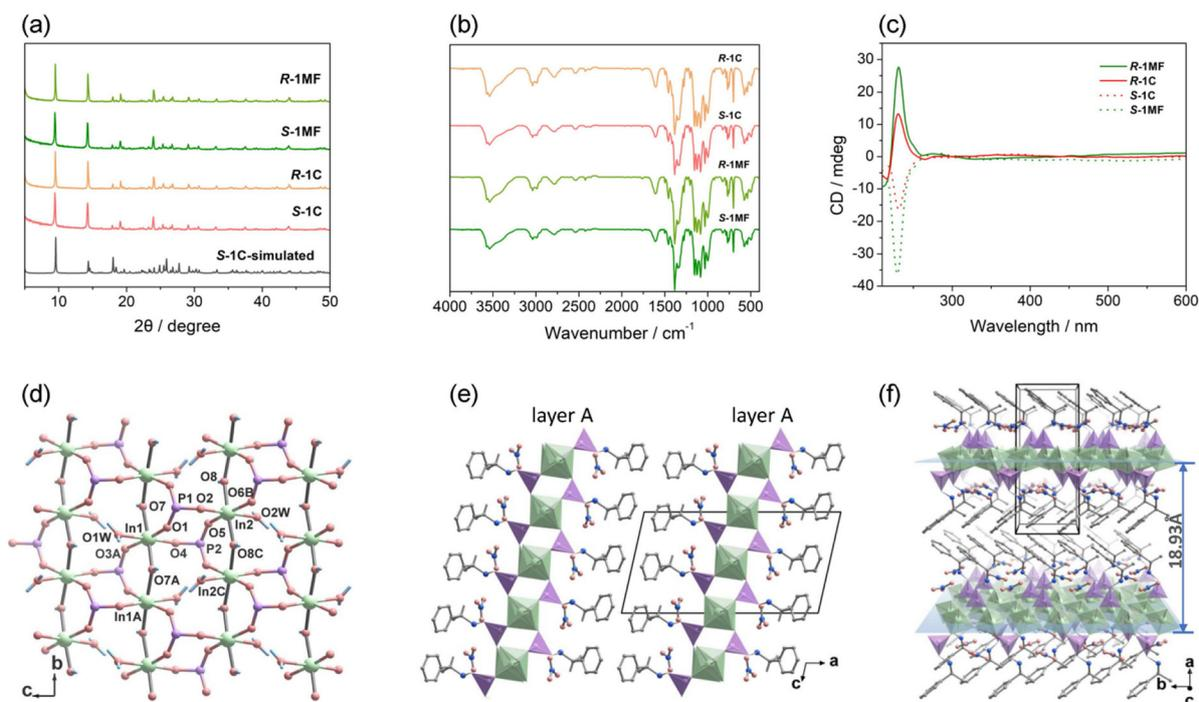
**Fig. 1** (a) PXRD patterns of the as-synthesized compounds *R*-, **S-1C** and *R*-, **S-1MF**. The pattern simulated from the single-crystal data of **S-1C** is given for comparison. (b) The IR spectra of *R*-, **S-1C** and *R*-, **S-1MF**. (c) Solid-state CD spectra of *R*-, **S-1C** and *R*-, **S-1MF**. (d) The inorganic layer of **S-1C**. (e) Packing diagram of **S-1C** viewed along the *b*-axis. (f) Packing diagram of **S-1C** viewed along the *c*-axis.
