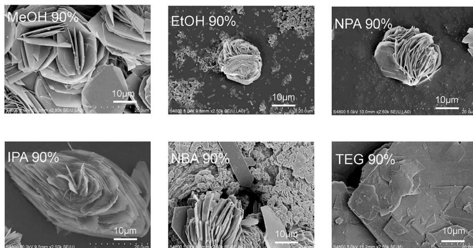
Fig. 3 SEM images of the self-assembled products of  $\text{In}(\text{NO}_3)_3$ / $S$ -pempH<sub>2</sub> in 90 vol% alcohol/H<sub>2</sub>O at 100 °C.
