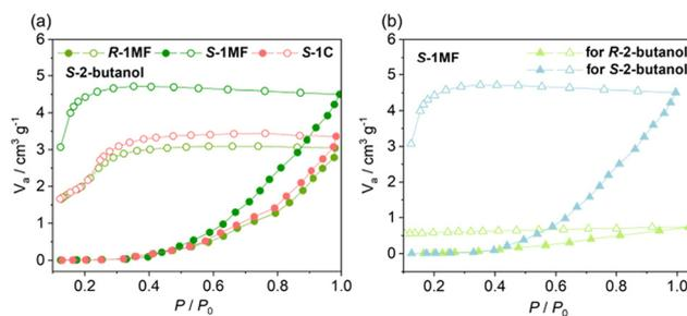
Fig. 6 (a) Comparison of the *S*-2-butanol adsorption (filled)/desorption (open) isotherms for the activated compounds *R*-1MF, *S*-1MF, and *S*-1C. (b) *S*- and *R*-2-butanol adsorption (filled) and desorption (open) isotherms for the activated compound *S*-1MF at 298 K.
