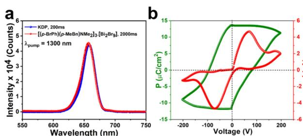
Fig. 2 (a) Comparison of the SHG emission profiles of [BPMBDMA]·[Bi<sub>2</sub>Br<sub>9</sub>] and the reference KDP sample. (b)  $P$ - $E$  hysteresis loop for [BPMBDMA]·[Bi<sub>2</sub>Br<sub>9</sub>] at room temperature.
