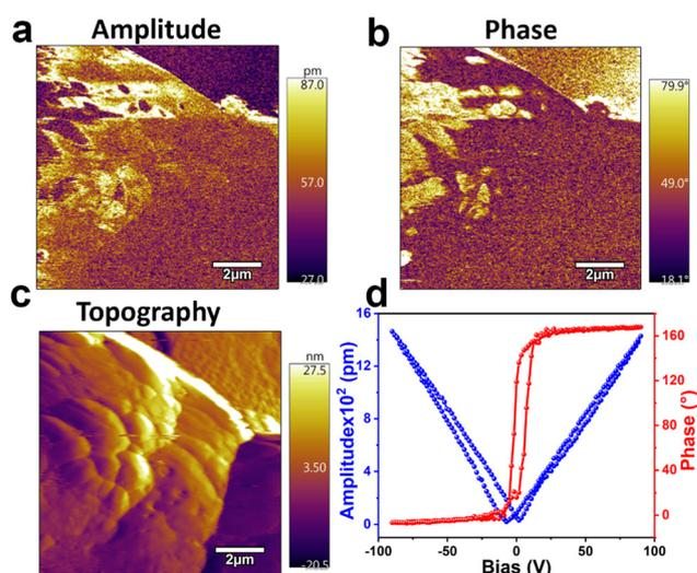
Fig. 3 PFM-derived (a) amplitude image and (b) phase image. (c) Topography of [BPMBDMA]·[Bi<sub>2</sub>Br<sub>9</sub>]. (d) Amplitude-bias "butterfly" (blue) and phase-bias "hysteresis" (red) loops of [BPMBDMA]·[Bi<sub>2</sub>Br<sub>9</sub>].
