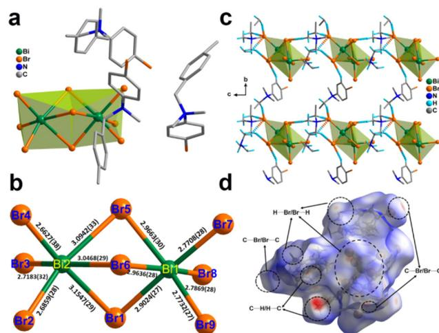
**Fig. 1** (a) Asymmetric unit of  $[\text{BPMBDMA}]\cdot[\text{Bi}_2\text{Br}_9]$ . (b) Bi-octahedral  $\text{Bi}_2\text{Br}_9$  unit with Bi and Br bond distances. (c) C-H...Br H-bonding interactions present in  $[\text{BPMBDMA}]\cdot[\text{Bi}_2\text{Br}_9]$ . The phenyl rings are omitted for clarity. (d)  $d_{\text{norm}}$ -mapped HS showing different interactions present in  $[\text{BPMBDMA}]\cdot[\text{Bi}_2\text{Br}_9]$ .
