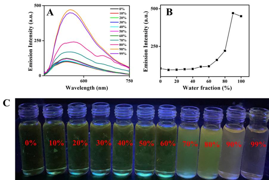
Fig. 4 (A) Emission spectra of 10 in different water fractions in THF and water mixture;  $\lambda_{\text{ex}} = 420$  nm. (B) Plots of emission intensity vs. water fraction. (C) Images of compound 9 in THF–water mixture with different water fractions (under UV light).
