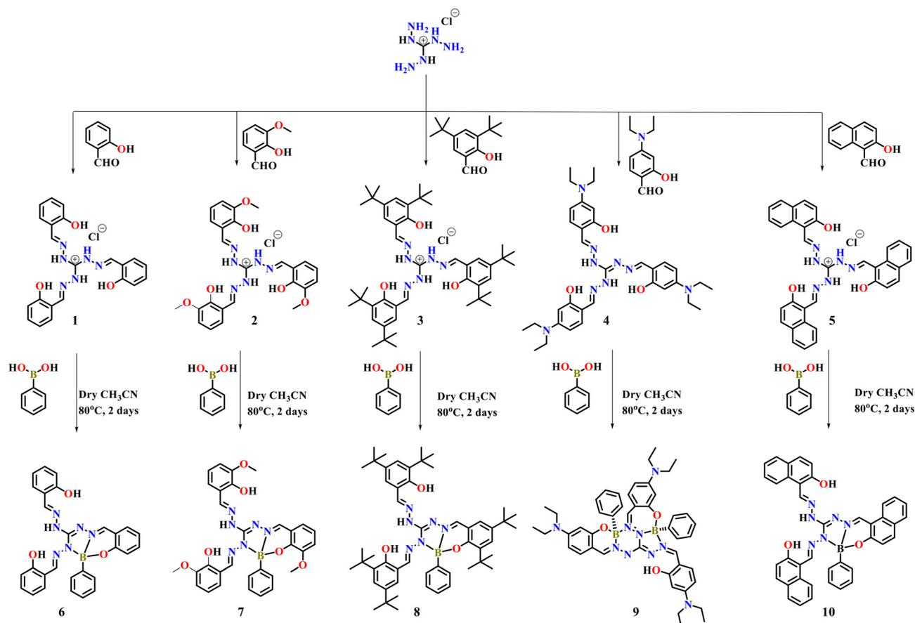
**Scheme 1** Synthesis of organoboron complexes **6–10** from triaminoguanidine-salicylidene Schiff bases (**1–5**).
