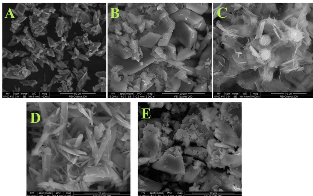
Fig. 5 (A) FESEM images of aggregates of compound 6 in 90% THF–H<sub>2</sub>O mixtures, (B) FESEM images of aggregates of compound 7 in 90% THF–H<sub>2</sub>O mixtures, (C) FESEM images of aggregates of compound 8 in 70% THF–H<sub>2</sub>O mixtures, (D) FESEM images of aggregates of compound 9 in 90% THF–H<sub>2</sub>O mixtures and (E) FESEM images of aggregates of compound 10 in 90% THF–H<sub>2</sub>O mixtures.
