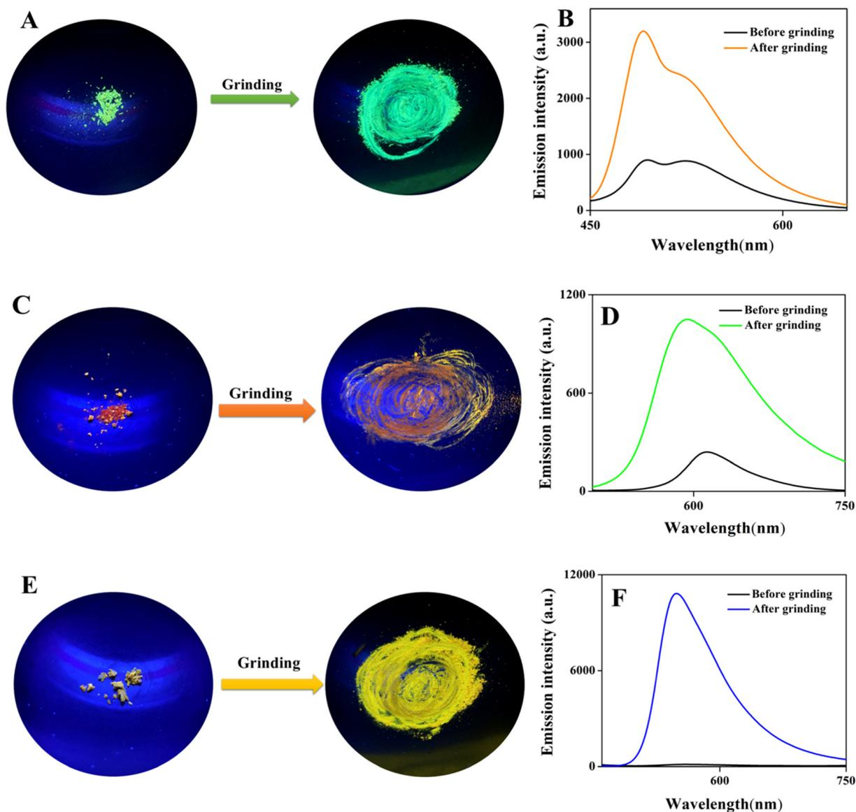
**Fig. 6** (A, C and E). Images of the boron compounds (**6**, **9** & **10**) before and after grinding under UV-lamp. (B, D, and F) Solid state emission spectra of compounds (**6**, **9** & **10**) crystals and ground samples.
