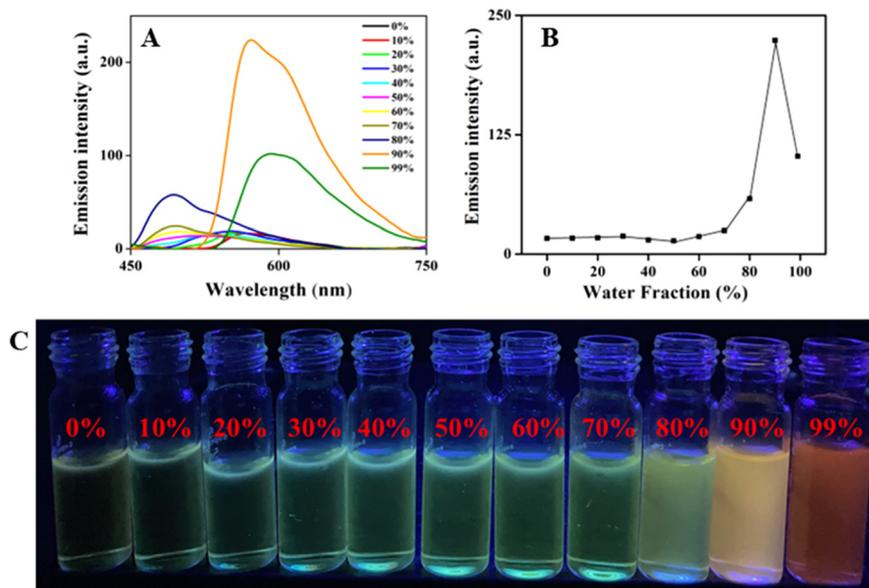
**Fig. 3** (A) Emission spectra of **9** in different water fractions in THF and water mixture;  $\lambda_{\text{ex}} = 420$  nm. (B) Plots of emission intensity vs. water fraction. (C) Images of compound **9** in THF–water mixture with different water fractions under UV light.
