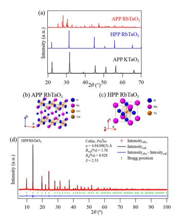
Fig. 1 (a) Powder XRD patterns ( $\lambda = 1.5418$  Å) of the APP and HPP of RbTaO<sub>3</sub>, and KTaO<sub>3</sub>, (b) the crystal structure models of the APP of RbTaO<sub>3</sub>, (c) the HPP of RbTaO<sub>3</sub>, and (d) Rietveld analysis ( $\lambda$  = 0.690388 Å) of the HPP of RbTaO<sub>3</sub>.  $R_{wp} = 1.57\%$  and S = 2.53.
