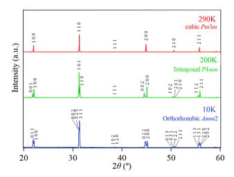
Fig. 3 XRD patterns and Miller indices of the three phases in the HPP of RbTaO<sub>₹</sub>.
