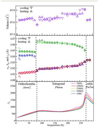
Fig. 4 Temperature dependence of lattice parameters, volume, and relative permittivity of a bulk disk, which has an 88% packing density, of RbTaO<sub>3</sub> at 4-280 K.  $a_p$ ,  $b_p$ ,  $c_p$ , and v are taken from a basic perovskite
