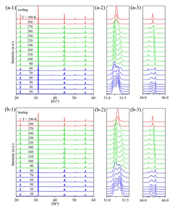
Fig. 2 Powder XRD patterns of the HPP of RbTaO<sub>3</sub> at 290–10 K (a) in the cooling process ((a-1) overall view, (a-2) 110 diffraction peak of the cubic phase, (a-3) 200 diffraction peak of the cubic phase) and (b) in the heating process, (b-1), (b-2) and (b-3) are same range. Red, green, and blue indicate cubic, tetragonal, and orthorhombic structures, respectively.
