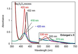
Fig. 8 UV-visible spectra of 6 μM solutions of the [Fe<sup>III</sup>TPPS/ Cu<sup>II</sup>BipyCD<sub>2</sub>] complex (green line), its reduced Fe<sup>II</sup>/Cu<sup>I</sup> (black line), oxygenated Fe<sup>III</sup>-O<sub>2</sub>·-/Cu<sup>I</sup> (blue line) and carboxylated Fe<sup>II</sup>-CO/Cu<sup>I</sup> (red line) products in 0.05 M phosphate buffer at pH 7. The inset shows an enlargement of the Q-band region.
