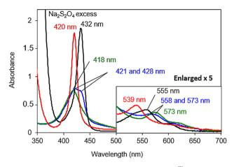
Fig. 7 UV-visible spectra of 8  $\mu$ M solutions of the [Fe<sup>III</sup>TPPS/BipyCD<sub>2</sub>]<sup>-</sup> complex (green line), its reduced Fe<sup>II</sup> (black line), oxygenated Fe<sup>III</sup>-O<sub>2</sub>. (blue line) and carbonylated Fe<sup>II</sup>-CO (red line) products in 0.05 M phosphate buffer at pH 7. The inset shows an enlargement of the Q-band
