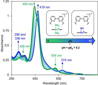
Fig. 3 UV-visible spectral changes of Fe<sup>III</sup>TPPS/BipyCD<sub>2</sub> (10 μM) in aqueous 0.1 M NaClO<sub>4</sub> as a function of the pH of the solution from 2 to 12. The pH was adjusted by addition HClO<sub>4</sub> and NaOH.
