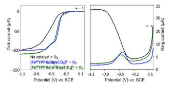
Fig. 9 Voltammograms measured by RRDE experiments of the various complexes (10  $\mu$ L of a 2.5 mM solution) coated with Nafion (10  $\mu$ L) on the disk electrode in  $O_2$ -saturated solution, measured at pH 7 in 0.05 M phosphate buffer containing 0.5 M Na<sub>2</sub>SO<sub>4</sub> at a scan rate of 0.02 V s<sup>-1</sup> and 100 rpm.
