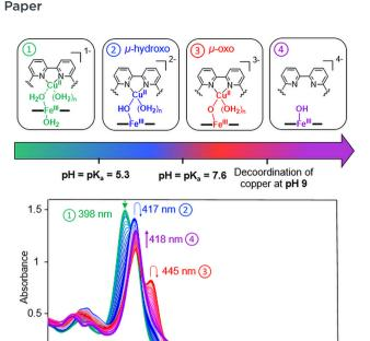
Fig. 5 UV-visible spectral changes of  $[Fe^{III}TPPS/Cu^{II}BipyCD_2]$  (14  $\mu$ M) in aqueous 0.1 M NaClO<sub>4</sub> as a function of the pH of the solution from 2 to 12. The pH was adjusted by addition HClO<sub>4</sub> and NaOH.
