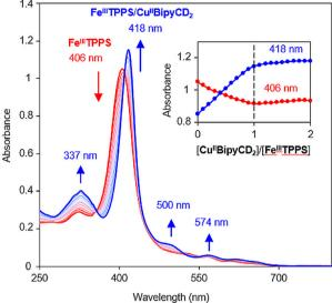
Fig. 4 UV-visible titration of Fe<sup>III</sup>TPPS (10 µM) in 0.05 M phosphate buffer with the stepwise addition of Cu<sup>II</sup>BipyCD<sub>2</sub> in water. The inset shows changes in absorbance as a function of ratio of the concentrations [Cu<sup>II</sup>BipyCD<sub>2</sub>]/[Fe<sup>III</sup>TPPS].
