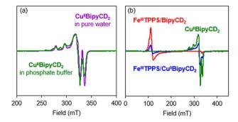
Fig. 6 EPR spectra at 25 K of (a)  $[Cu^{II}BipyCD_2]^{2+}$  (0.5  $\mu$ M) in water (purple line) or in 0.025  $\mu$ M phosphate buffer at pH 7 (green line) and (b)  $[Fe^{III}TPPS/BipyCD_2]^{3-}$  (red line),  $[Cu^{II}BipyCD_2]^{2+}$  (green line) and  $[Fe^{III}TPPS/Cu^{II}BipyCD_2]^{-}$  (blue line) in 0.025 phosphate buffer at pH 7.
