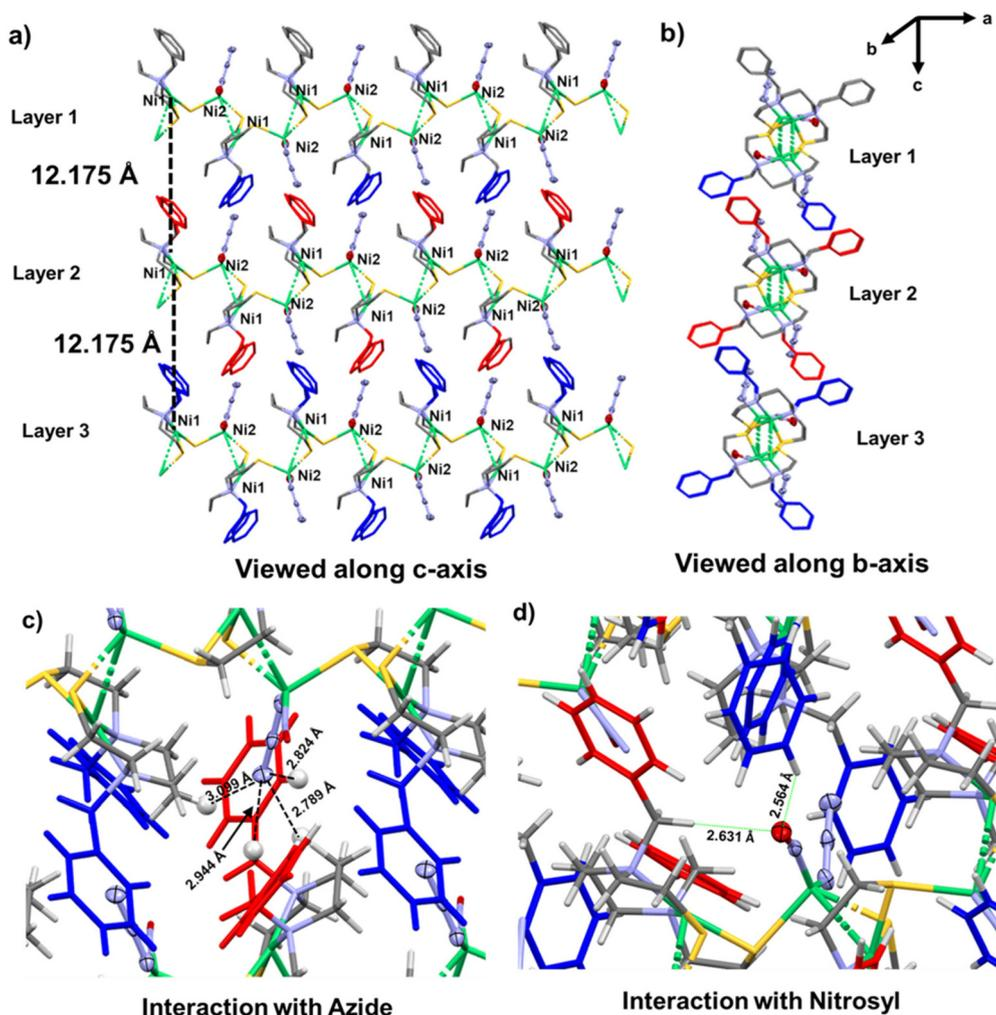
**Fig. 3** (a) Three layers of complex 2 viewed along *c*-axis. The distance between the Ni centers in two layers is 12.175 Å. (b) Three layers of complex 2 viewed along *b*-axis. (c) Zoomed in view of the interaction between the azide group and the aliphatic and aromatic hydrogens. (d) Zoomed in view of the interaction between nitrosyl group and aliphatic and aromatic hydrogens.
