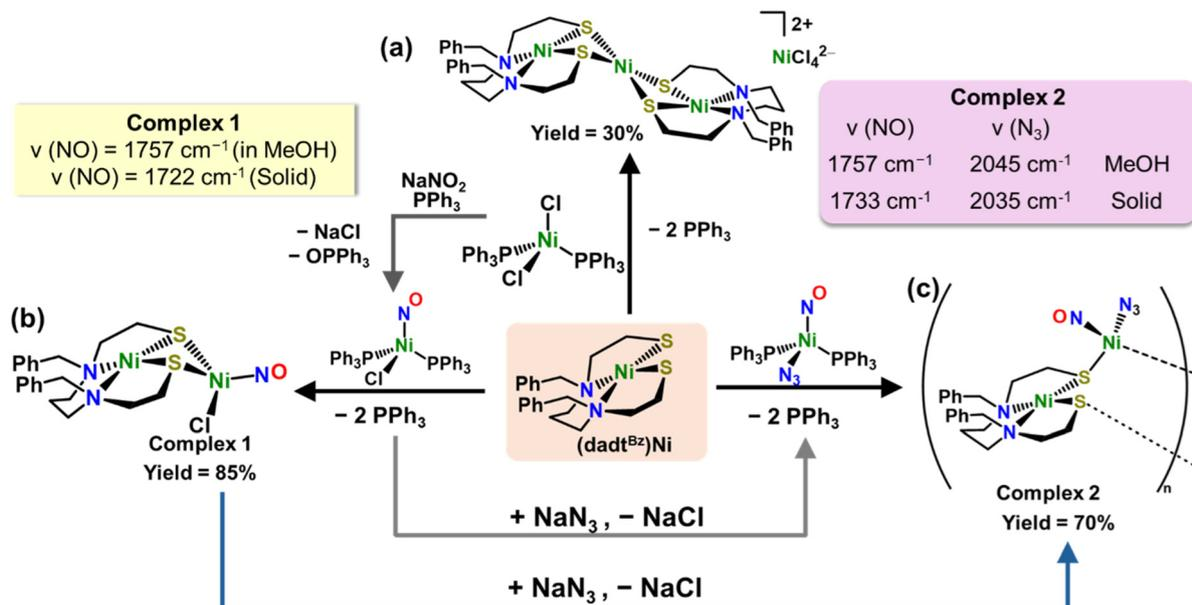
**Scheme 1** Synthetic routes to complexes reported in this study. MeOH was used as a solvent for all reactions. Note: complex 2 is the coordination polymer, alternatively referred to as CP2.
