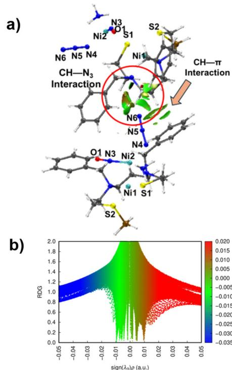
**Fig. 6** (a) NCI index on the unit cell of complex 2 using iso surface value of 0.5 au and the color scale is  $-0.05 < \rho < 0.05 \text{ au}$ . CH- $\pi$  interactions are shown with arrow and the red circle indicates the CH-N<sub>3</sub> interaction. (b) Reduced density gradient plot shows prominent attractive interactions in complex 2.
