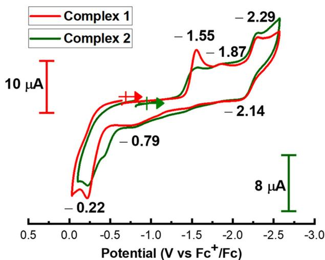
**Fig. 4** Cyclic voltammetry of complex 1 (red) and complex 2 (green) in DMF containing a 0.1 M [ $^t\text{Bu}_4\text{N}$ ][PF $_6$ ] electrolyte and 2.0 mM complex at room temperature. Note that complex 2 has poor solubility in DMF, leading to reduced current intensity during the cyclic voltammetry analysis.
