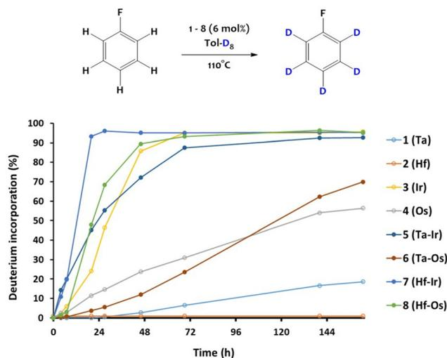
**Fig. 3** Kinetic monitoring of fluorobenzene deuteration in toluene-*d*<sub>8</sub> at 110 °C using complexes **1–8** as catalysts (6 mol%).
