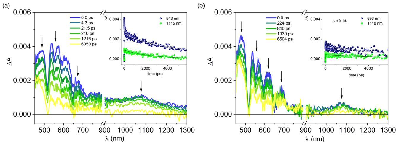
**Fig. 7** Transient absorption spectra of **P-Pyr<sub>4</sub>@(Rucage)<sub>4</sub>** (a) and **P-Pyr<sub>4</sub>** (b) in DCM at different delays. Excitation at 420 nm ( $A_{420} = 0.20$ , 0.2 cm optical path, 1  $\mu\text{J}$  per pulse). Inset:  $\Delta A$  time evolutions (dots) and fittings (lines) at the indicated wavelengths.
