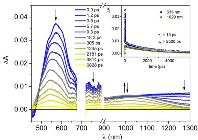
**Fig. 6** Transient absorption spectra of **P-Pyr<sub>4</sub>@(Rucage)<sub>4</sub>** in DCM at different delays. Excitation at 700 nm ( $A_{700} = 0.34$ , 0.2 cm optical path, 10  $\mu$ J per pulse). Inset:  $\Delta A$  time evolutions (dots) and fittings (lines) at the indicated wavelengths.
