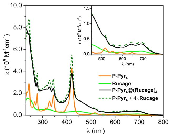
**Fig. 4** Absorption spectra of **P-Pyr<sub>4</sub>@(Rucage)<sub>4</sub>** and its respective models **P-Pyr<sub>4</sub>** and **Rucage** in DCM. The weighted sum of the spectra of the models is also reported. Inset: magnification of the 450–800 nm region.
