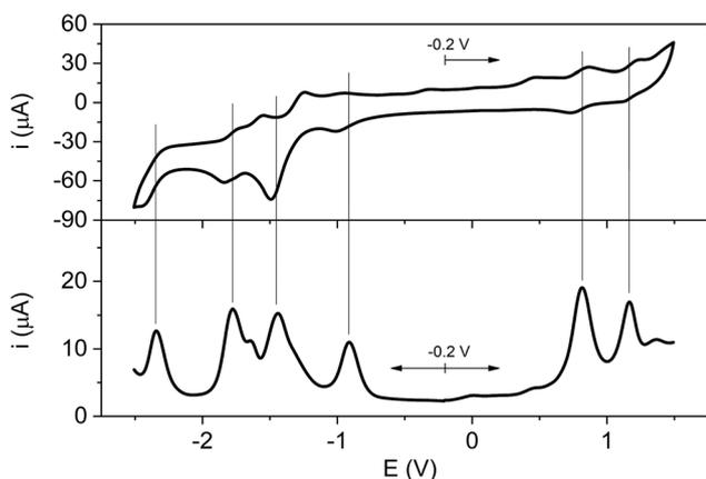
**Fig. 3** Cyclic (top panel) and square wave (bottom panel) voltammetry scans of **Rucage** in DCM solution. CV anodic scan starting from  $-0.2 \text{ V}$ ; SWV anodic and cathodic scans from  $-0.2 \text{ V}$  (the sign of the cathodic current is reversed).
