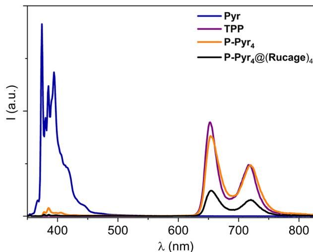
**Fig. 5** Corrected emission spectra of isoabsorbing solutions of **P-Pyr<sub>4</sub>**, **P-Pyr<sub>4</sub>@(Rucage)<sub>4</sub>** and models **Pyr** and **TPP** in DCM; excitation at 345 nm ( $A_{345} = 0.11$ ); at this wavelength the pyrenyl units are almost exclusively excited (90% of the absorbed photons).
