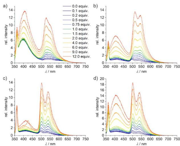
**Fig. 4** Emission spectra of (a) [Pt(A)(<sup>Cl</sup>L<sup>Cl</sup>)] and (b) [Pt(A)(<sup>Cl</sup>L)] upon stepwise addition of *c-myc22* (0–12 equiv.). Emission spectrum of [Pt(B)(<sup>OH</sup>L)]OTf upon stepwise addition of (c) *c-kit* and (d) H-Telo (0–12 equiv.). Conditions: metal complex (1  $\mu\text{M}$ ), LiCl (90 mM), KCl (10 mM), MOPS (5 mM, pH 7.4), 20 °C,  $\lambda_{\text{exc}} = 340$  nm.
