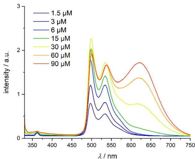
Fig. 3 Concentration-dependent emission spectra of  $[\text{Pt}(\text{A})(\text{M}^{\text{L}})]$ . Conditions: metal complex (1.5–90  $\mu\text{M}$ ), 20  $^{\circ}\text{C}$ ,  $\lambda_{\text{exc}} = 340 \text{ nm}$ .
