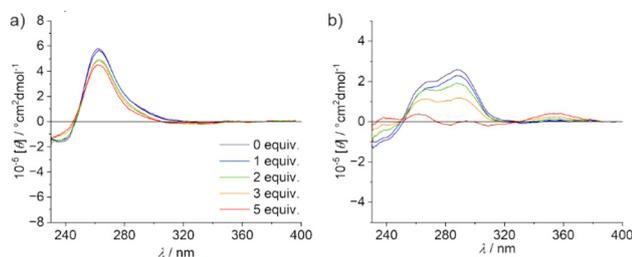
**Fig. 5** CD spectra of (a) *c-myc22* upon stepwise addition of [Pt(B)<sup>(ML)</sup>]OTf and (b) *bcl2-mid* upon stepwise addition of [Pt(B)<sup>(PL)</sup>]OTf (0–5 equiv.). Conditions: DNA (3 μM), LiCl (90 mM), KCl (10 mM), MOPS (5 mM, pH 7.4), 20 °C.
