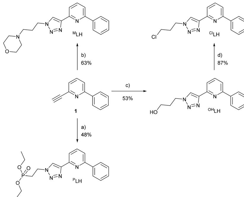
**Scheme 1** a) Diethyl (2-azidoethyl)phosphonate, general procedure for click reaction; (b) 4-(3-azidopropyl)morpholine, general procedure for click reaction; (c) 3-azidopropan-1-ol, general procedure for the click reaction; (d)  $SOCl_2$ ,  $CH_2Cl_2$ ,  $0^\circ C$ , o/n.
