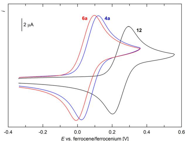
**Fig. 5** Cyclic voltammograms of **4a**, **6a**, and **10** as recorded on a glassy carbon disc electrode in  $\text{CH}_2\text{Cl}_2$  (0.1 M  $\text{Bu}_4\text{N}[\text{PF}_6]$ , scan rate  $100 \text{ mV s}^{-1}$ ).
