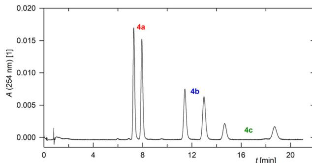
**Fig. 1** SFC chromatogram of an equimolar **4a–4c** mixture (Lux® i-Amylose-3 column, 150 × 4.6 mm, particle size 3 μm, CO<sub>2</sub>-methanol 80:20, 2 mL min<sup>-1</sup>, 40 °C, back pressure regulator 2000 psi, UV detection at 254 nm).
