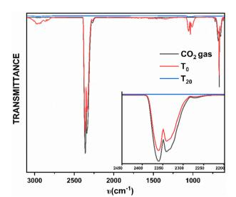
Fig. 2 The comparative gas-phase IR spectra of free  $CO_2$  gas (black), headspace of the reaction mixture in the beginning ( $T_0$ , red) and headspace of the reaction mixture after 20 minutes ( $T_{20}$ , blue).
