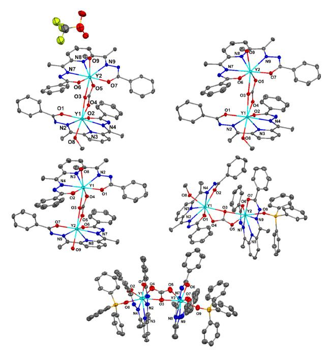
Fig. 3 ORTEP representations with 40% ellipsoid probability for the solid-state single crystal X-ray molecular structures of 1·Y (top left), 2·Y (top right), 3·Y (middle left), 5·Y (middle right), and 6·Y (bottom). The atomic sites of the inner coordination environments are labelled. The H atoms and the co-crystallized solvent molecules are omitted for clarity. Color codes: cyan, Y; yellow, S; orange, P; greenish yellow, F; red, O; blue, N; and grey, C.
