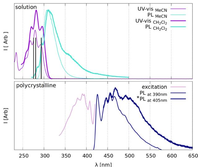
**Fig. 2** Top: normalized UV-vis and PL spectra of ArPET in solution with TDDFT-predicted electronic excitations represented as vertical black lines. Bottom: excitation and PL spectra from crystalline ArPET-I.
