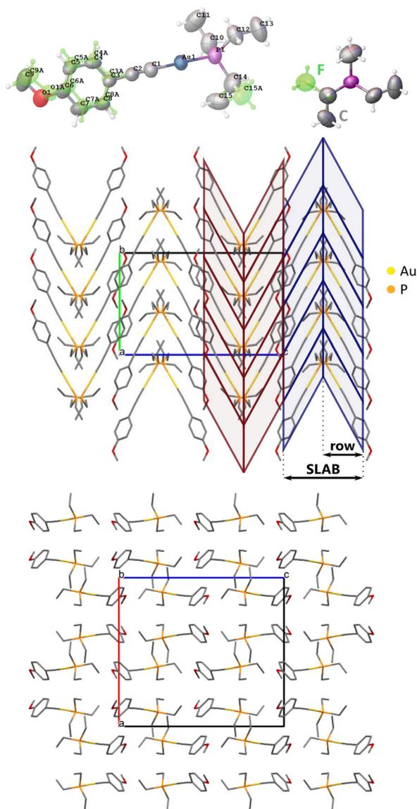
**Fig. 3** Structure of ArPEt at 295 K and under ambient pressure with its atom numbering scheme (upper left). The green part refers to the minor fraction of disorder; atomic displacement parameters represented at a 50% probability level; and triethylphosphine conformations in disordered variants (upper right). Herringbone-like motif in the crystal structure of ArPEt: view along the [100] direction highlighting the most important packing motifs (middle) and view along [010] (down).
