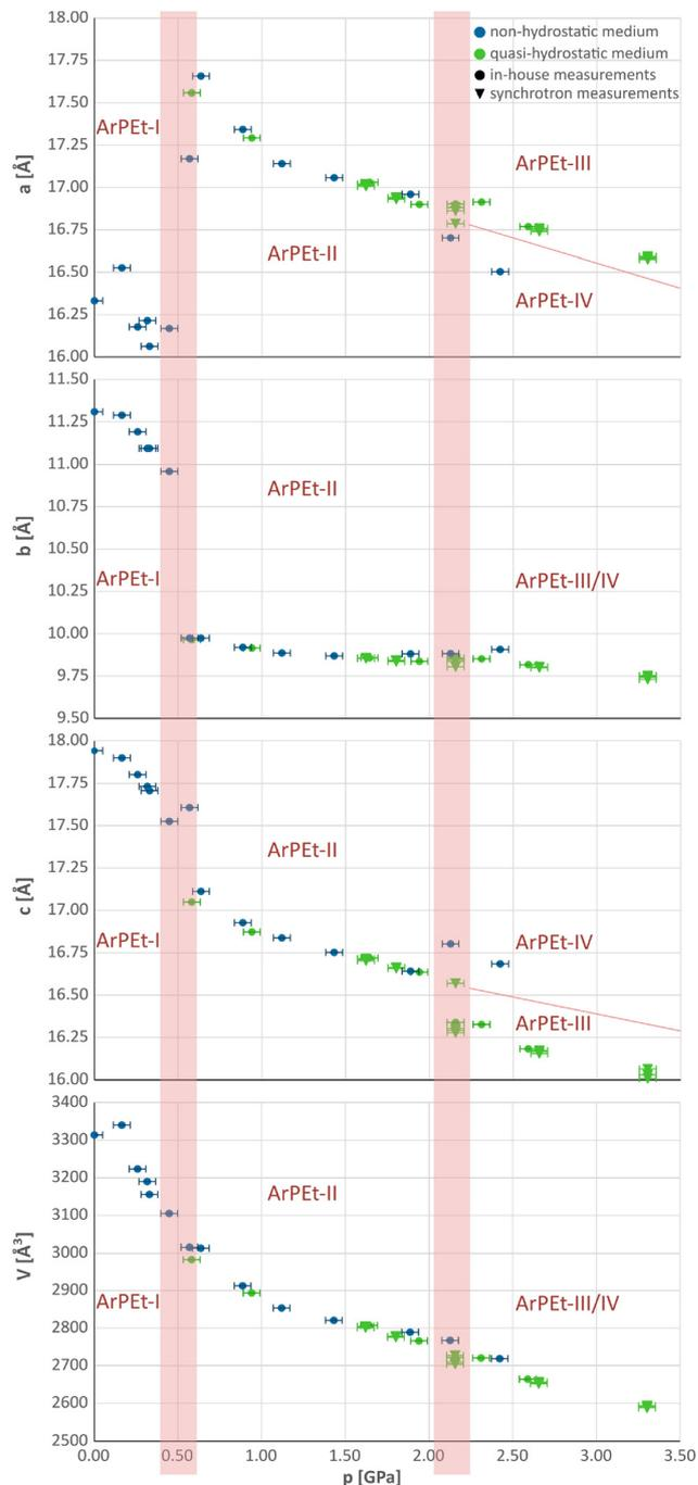
**Fig. 4** Evolution of the unit cell parameters with pressure in crystalline ArPEt based on the in-house and synchrotron measurements. Silicone oil is marked as a non-hydrostatic medium (blue), while the  $n$ -pentane/ $i$ -pentane 1:1 mixture and Daphne-7575 are marked as quasi-hydrostatic media (green). Uncertainties of pressures approximated as 0.05 GPa; experimental uncertainties of unit cell parameters are smaller than the drawn points.
