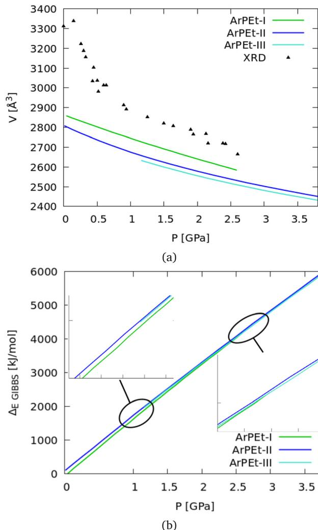
**Fig. 8** (a) Theoretical (solid lines) and experimental (SC-XRD) unit cell volumes as a function of pressure; theoretical predictions are noticeably underestimated; (b) theoretically predicted enthalpies for the selected ArPET polymorphs; the three curves approach each other at about 2.7 GPa.
