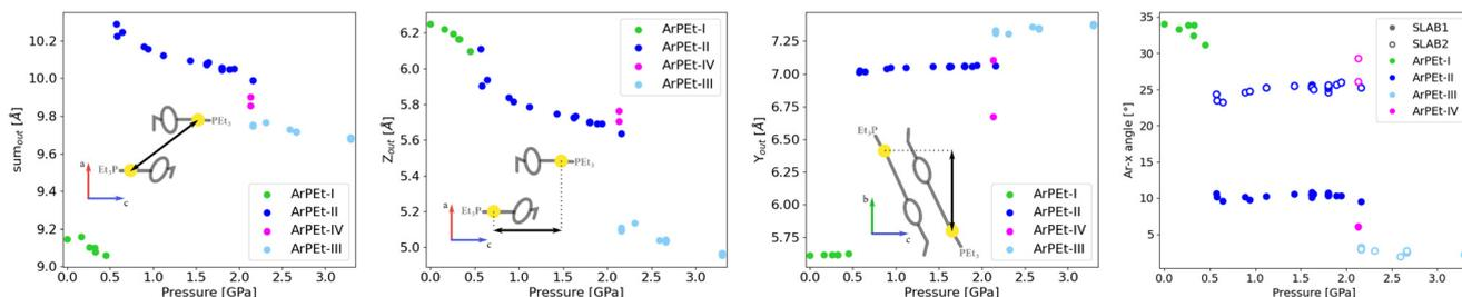
**Fig. 5** Calculated distances between neighboring gold atoms – overall (first), along [001] (second) and along [010] (third). The angle between aryl moieties and [100] in the unit cell (fourth). Definitions of distances are given in section S5 in the ESI<sup>†</sup>
