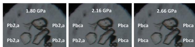
**Fig. 10** Four crystal specimens of ArPET as placed inside a DAC during X-ray diffraction experiments at the ESRF. Space groups at which data were indexed for each specimen at a given pressure indicate a particular ArPET phase. A piece of gold foil (dark triangle) and ruby spheres are visible in the lower-right corner.
