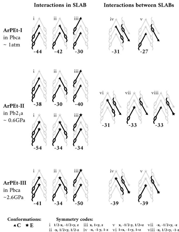
**Fig. 9** Definition of the dimers in SLABs (interaction energy  $>20 \text{ kJ mol}^{-1}$ ) and interaction energies  $[\text{kJ mol}^{-1}]$  calculated for subsequent dimers on a schematic representation of ArPET crystal packing along the  $[100]$  direction.
