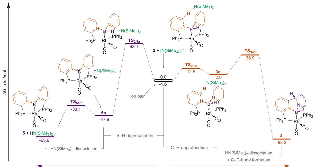
**Fig. 5** Calculated possible pathways for the deprotonation of **2**. Left: The deprotonation at the boron leads to a boride species **5** via  $\text{HN}(\text{SiMe}_3)_2$ -stabilised intermediate **5a**. Right: The deprotonation at position 6 at the pyridine ring results in  $\text{HN}(\text{SiMe}_3)_2$ -stabilised intermediate **3a**, followed by dissociation and C–C-bond formation leading to **3** ( $\Delta G$  values are given in  $\text{kJ mol}^{-1}$ ).
