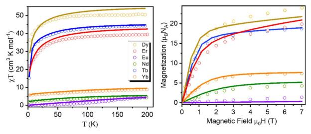
Fig. 11 (Left) Thermal dependence of the molecular magnetic susceptibility for Ln<sub>4</sub> complexes. The simulated results are scaled up by 3% in order to make it compatible with experimental data. (Right) Magnetization (M) versus magnetic field (H) plot for all the complexes at 2 K. The circles indicate the experimental values, while the lines represent the POLY\_ANISO-simulated data.
