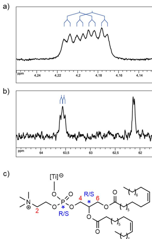
**Fig. 5** (a and b) Sections of 1D NMR spectra of solution **B** in  $\text{DMSO}-d_6$ , exhibiting a splitting of some of the signals of complex **3**. (a)  $^1\text{H}$  NMR (500 MHz): one of the H6 signals. (b)  $^{13}\text{C}\{^1\text{H}\}$  NMR (125 MHz): C4 and C6 signals (decreasing chemical shift). (c) The proposed partial formula for complex **3** with stereogenic centers and partial numeration of the protons and carbons.
