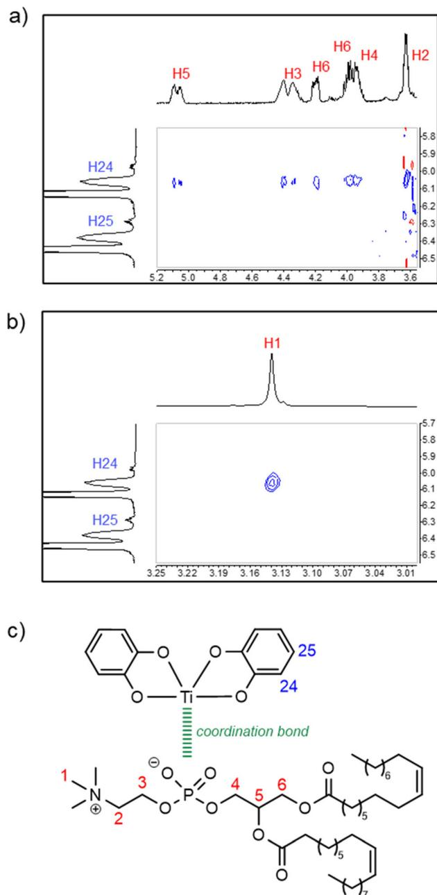
**Fig. 4** (a and b) Sections of the  $^1\text{H}$ - $^1\text{H}$  NMR ROESY spectrum of solution **B** in  $\text{DMSO}-d_6$  (500 MHz), exhibiting signals of complex **3**. (c) The proposed structural formula for complex **3**. The cross-peaks reveal a close spatial contact between one of the catechol protons (represented in blue) and the DOPC protons (represented in red).
