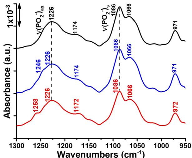
Fig. 1 ATR-FTIR spectra highlighting the interaction of titanium complexes 1 and 2 with DOPC multi-bilayers at room temperature. Black curve: spectrum of DOPC multi-bilayers hydrated with  $\text{H}_2\text{O}$ . Blue and red curves: spectra of complexes 1 and 2, respectively, inserted into DOPC multi-bilayers at a complex/lipid ratio of 1/20 and hydrated by  $\text{H}_2\text{O}$ .
