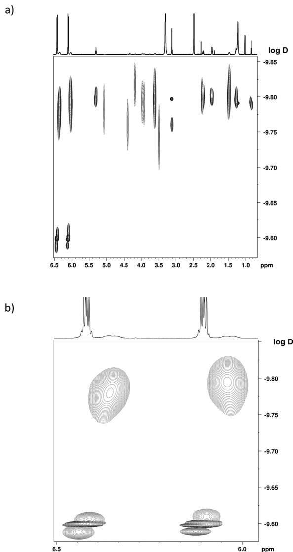
Fig. 3 <sup>1</sup>H NMR DOSY spectrum of solution **B**, exhibiting the signals of complexes **1** and **3** in DMSO-*d*<sub>6</sub> (600 MHz). (a) Section from 0.7 to 6.5 ppm. (b) Zoom on the catecholato signals.
