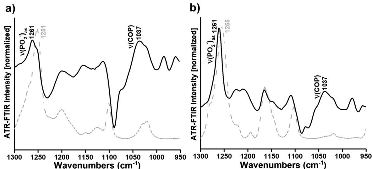
**Fig. 2** Gray dashed curves: ATR-FTIR spectra of complexes 1 and 2 as dry films from solutions in methanol (a and b, respectively). Black curves: difference ATR-FTIR spectra calculated by subtracting the spectrum of DOPC multi-bilayers from the spectra of complex 1/DOPC and complex 2/DOPC multi-bilayers (a and b). Both spectra in a and b were normalized to the same intensity for better visualization of the characteristic contributions of complexes 1 and 2 in the respective difference spectra.
