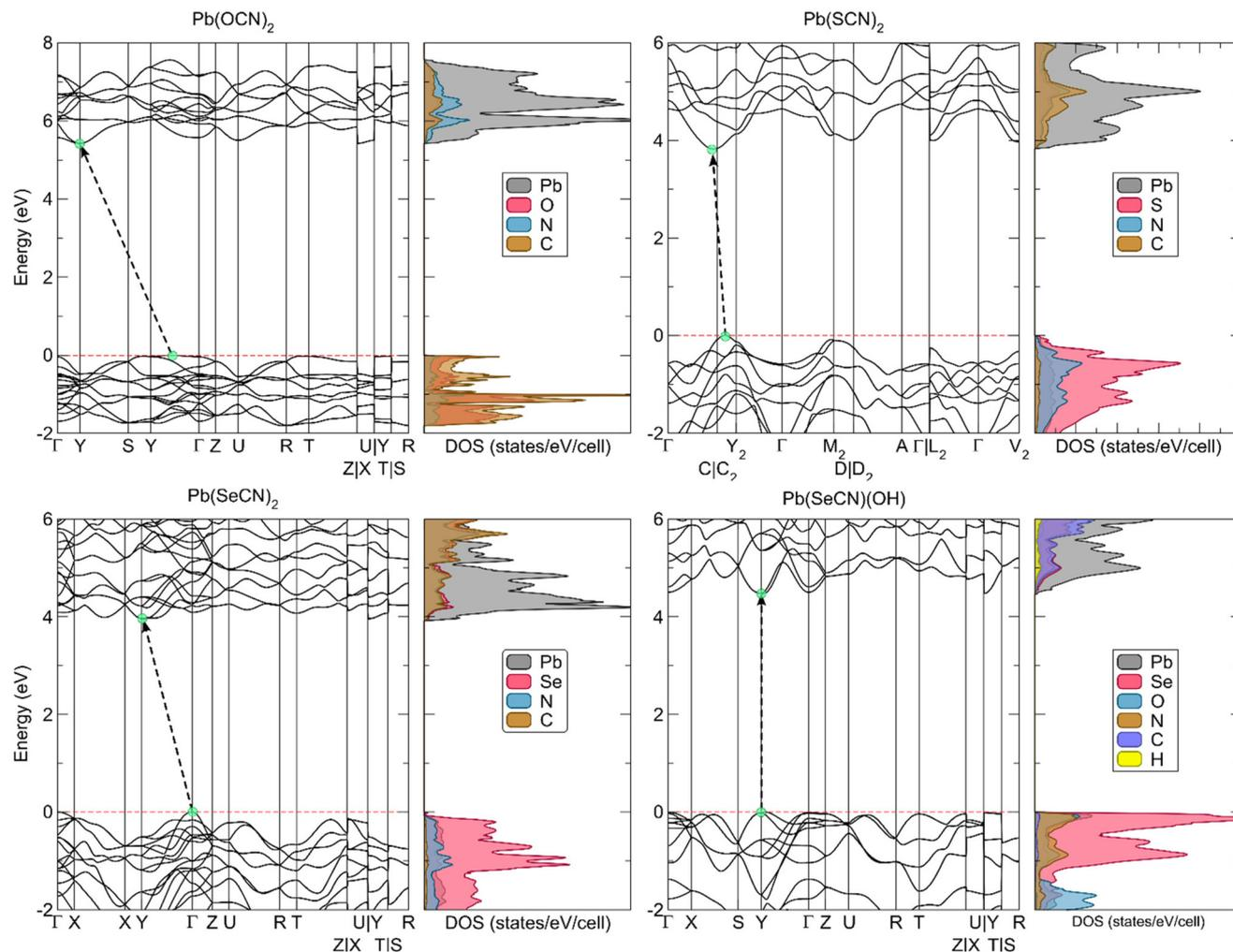
**Fig. 21** Electronic band structure together with atomic-projected electronic densities of states of the lead-based compounds under scrutiny. The black dashed arrows and teal circles indicate the fundamental band transition, while the red dashed line indicates the highest occupied crystalline orbital.
