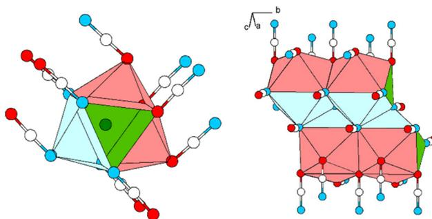
**Fig. 2** Excerpt of the crystal structure of Pb[OCN]<sub>2</sub>. Left: coordination polyhedron around Pb. Right: double-chain of polyhedra around Pb extending along [010]. Green: Pb, white: C, blue: N, red: O.
