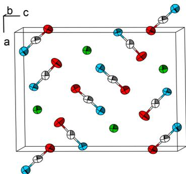
**Fig. 1** The crystal structure of Pb[OCN]<sub>2</sub>. Thermal displacement ellipsoids are drawn at the 75% probability level at 100 K. Green: Pb, white: C, blue: N, red: O.
