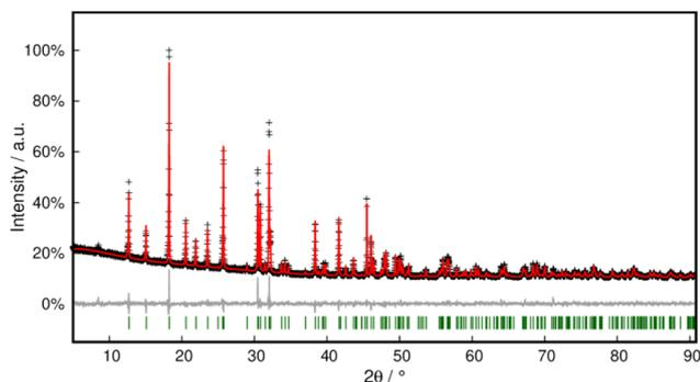
**Fig. 4** Rietveld refinement of  $\text{Pb}[\text{OCN}]_2$  at 298 K. Black crosses display measured data; the red line represents the refined model, green bars indicate Bragg positions and the grey line displays the difference plot. Further data are compiled in Table S3.†
