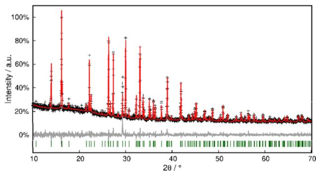
**Fig. 11** Rietveld refinement of  $\text{Pb}[\text{SeCN}]_2$  at 298 K. Black crosses display measured data; the red line represents the refined model, green bars indicate Bragg positions and the grey line displays the difference plot. Further data are compiled in Table S3.†
