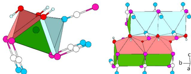
**Fig. 14** Excerpts from the crystal structure of  $\text{Pb}[\text{SeCN}][\text{OH}]$ . Left: coordination polyhedron around Pb (green) in the form of a distorted bicapped tetragonal antiprism, consisting of four Se, three O and one N atom. Right: double-chain of polyhedra stacked along [010]. Green: Pb, white: C, blue: N, magenta: Se, red: O, light blue: H.
