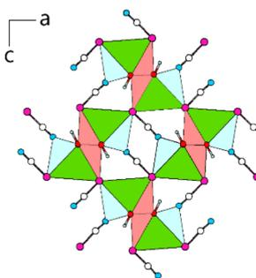
**Fig. 15** View along [010] of  $\text{Pb}[\text{SeCN}][\text{OH}]$ : double-chains of coordination polyhedra around Pb connected via common Se-vertices and  $[\text{SeCN}]^-$  anions. Green: Pb, white: C, blue: N, magenta: Se, red: O, light blue: H.
