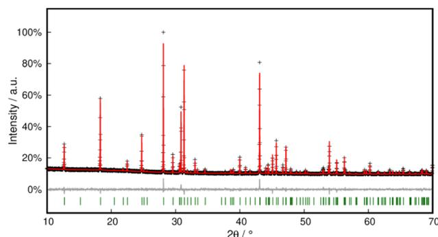
**Fig. 16** Rietveld refinement of  $\text{Pb}[\text{SeCN}][\text{OH}]$  at 298 K. Black crosses display measured data; the red line represents the refined model, green bars indicate Bragg positions and the grey line displays the difference plot. Further data are compiled in Table S3.†
