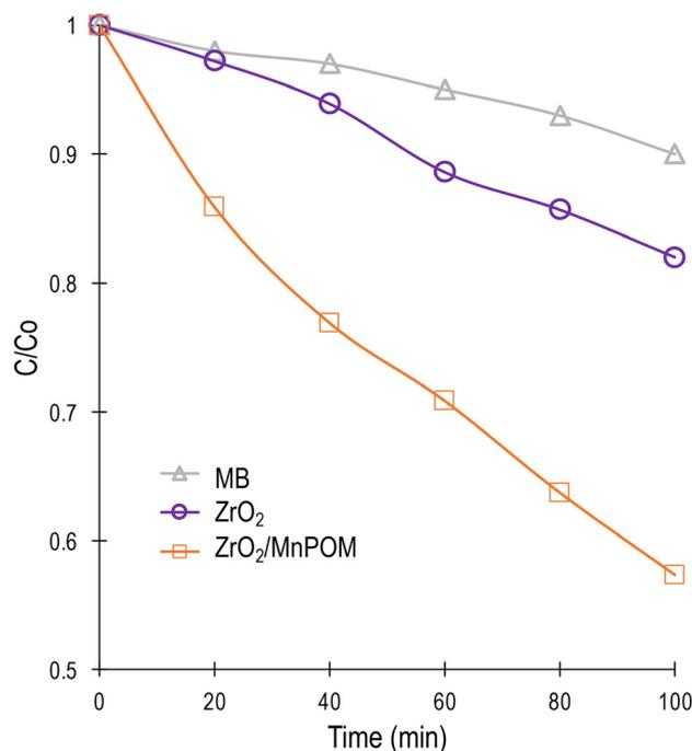
**Fig. 6** MB concentration decay under UV irradiation for free MB and onto bare ZrO<sub>2</sub> and ZrO<sub>2</sub>/MnPOM thin films.**Table 4** Photocatalytic efficiency of different systems under UV irradiation
