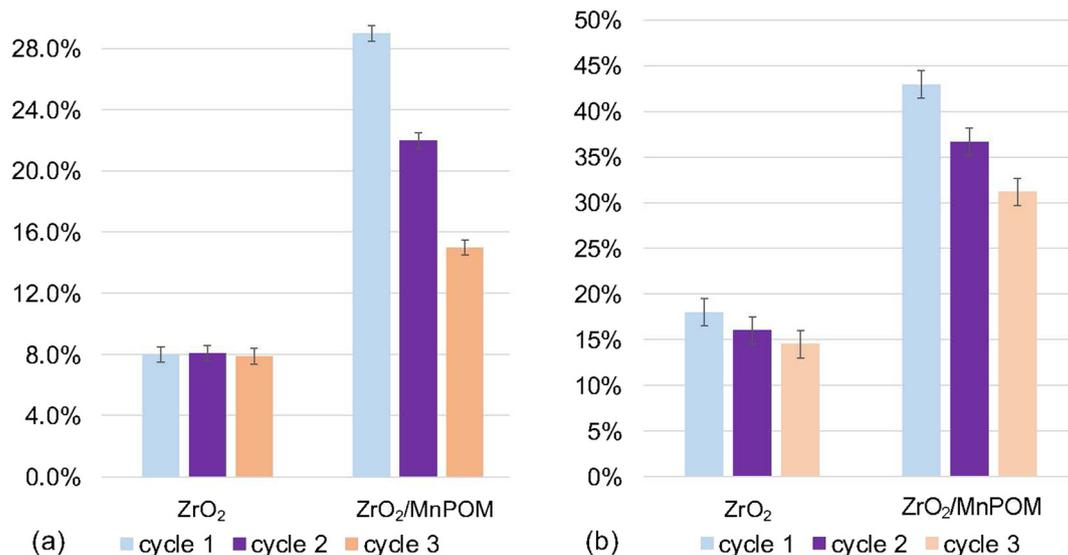
Fig. 7 Recyclability tests for photocatalytic degradation of MB onto ZrO<sub>2</sub> and ZrO<sub>2</sub>/MnPOM thin films. (a) Adsorption (b) photocatalytic degradation.
