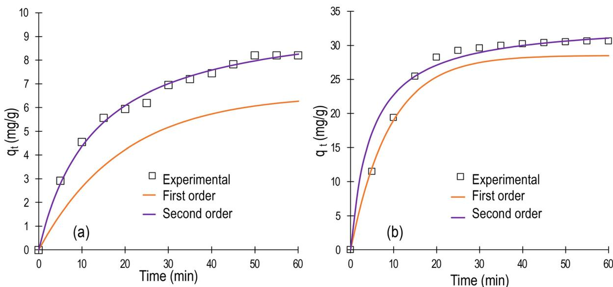
**Fig. 5** Kinetic fitting results of MB adsorption on both thin films: (a) ZrO<sub>2</sub> and (b) ZrO<sub>2</sub>/MnPOM.
