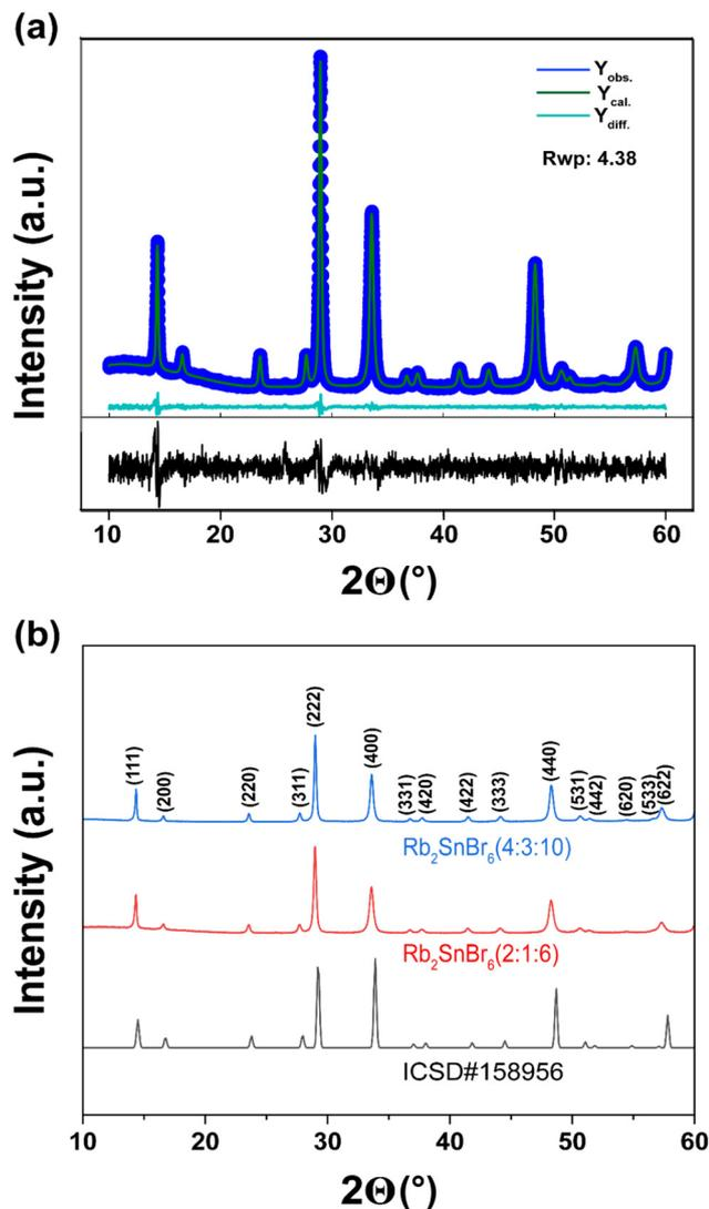
**Fig. 3** Analyzed powder XRD data: (a) Rietveld refinement plot of the  $\text{Rb}_2\text{SnBr}_6$  (4 : 3 : 10) double perovskite halide. Rietveld refinement data:  $Fm\bar{3}m$ ,  $a = 10.678 \text{ \AA}$ ,  $V = 1217.71 \text{ \AA}^3$ ,  $R_{\text{wp}} = 4.38\%$ , and (b) powder crystal XRD of  $\text{Rb}_2\text{SnBr}_6$  (2 : 1 : 6) and  $\text{Rb}_2\text{SnBr}_6$  (4 : 3 : 10), which are a close match to each other.
