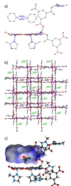
Fig. 7 (a) Structure of Azo@mDESY-1 at 290 K, counterions were omitted for clarity. (b) Packing of Azo@mDESY-1 at 290 K showing the position of the azobenzene molecule (green) in the channels of the MOF, counterions were omitted for clarity. (c) Hirshfeld isosurface of azobenzene inside of mDESY-1, showing the main interactions.
