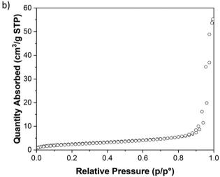
Fig. 6  $\rm\,N_2$  adsorption measurements at 77 K of (a) mDESY-1 and (b) mDESY-2.
