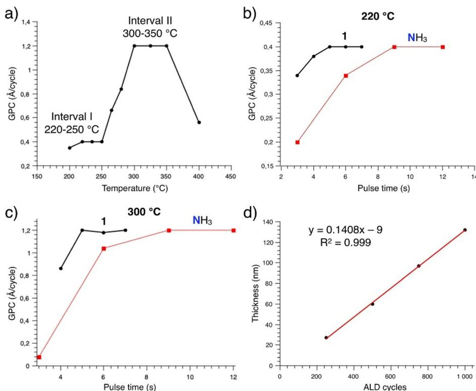
Fig. 3 ALD characteristics of the In(triaz)<sub>3</sub> with NH<sub>3</sub> plasma. (a) Dependence on growth per cycle (GPC) with process temperature, (b) saturation curves at 220 °C, (c) saturation curves at 300 °C, (d) film thickness as a function of number of ALD cycles. Reprinted from O'Brien *et al.*<sup>35</sup> under a CC-BY license.
