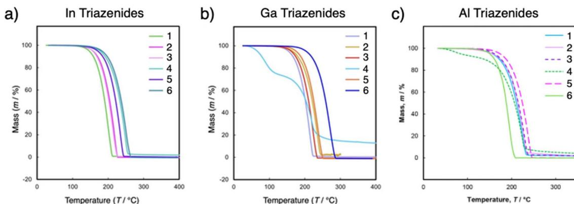
**Fig. 6** The TGA graphs from structural analogues (a) In triazenides, (b) Ga triazenides and (c) Al triazenides where 1 =  $\text{iPrN}_3\text{iPr}$ , 2 =  $\text{iPrN}_3\text{sBu}$ , 3 =  $\text{iPrN}_3\text{tBu}$ , 4 =  $\text{sBuN}_3\text{sBu}$ , 5 =  $\text{sBuN}_3\text{tBu}$  and 6 =  $\text{tBuN}_3\text{tBu}$ . Reprinted from Samii et al.<sup>41,42</sup> under a CC-BY license.
