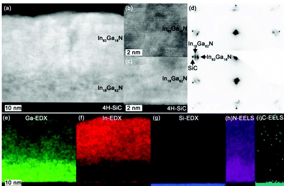
**Fig. 5** (a) cross-sectional STEM-HAADF image of the ~60 nm  $\text{In}_{1-x}\text{Ga}_x\text{N}$  film on the 4H-SiC substrate with a zoomed in image of the (b)  $\text{In}_{82}\text{Ga}_{18}\text{N}$  and (c)  $\text{In}_{18}\text{Ga}_{82}\text{N}$  layers. (d) SAED pattern from the film and substrate. EDX maps of (e) Ga, (f) In and (g) Si. EELS maps on (h) N and (i) C. Reprinted from Rouf et al.<sup>39</sup> under a CC-BY license.
