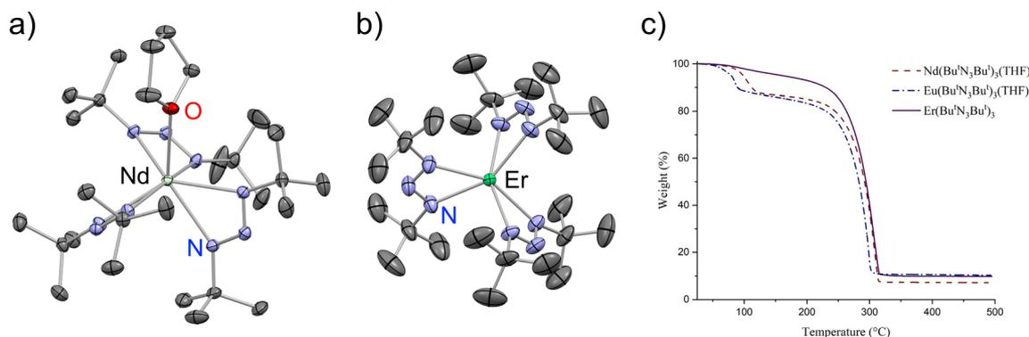
**Fig. 10** The crystal structure of (a) the Nd triazenide with a coordinated THF molecule and (b) the Er triazenide. (c) The TGA graphs of the lanthanide triazenides. Reprinted from Caroff and Girolami, Copyright 2022 American Chemical Society.<sup>49</sup>
