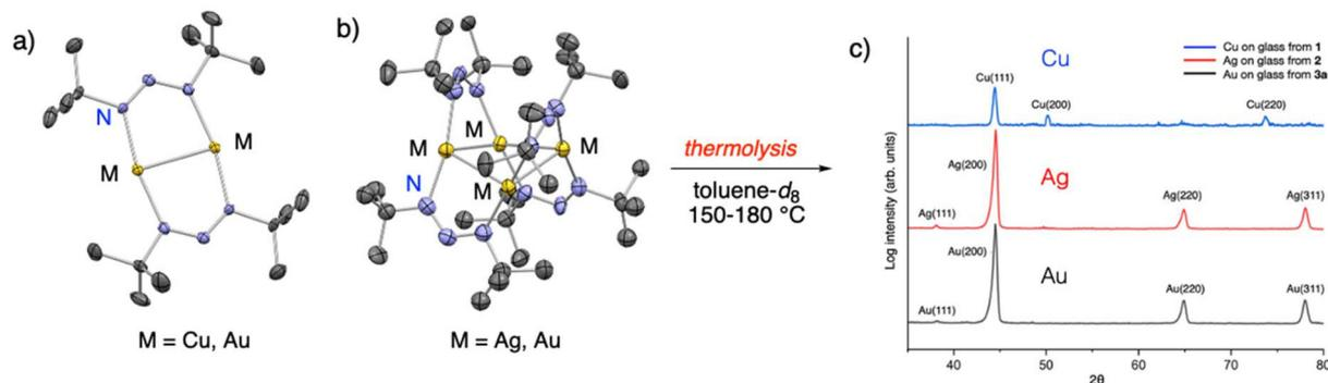
**Fig. 8** The crystal structure of (a) dinuclear Cu and Au, and (b) tetranuclear Ag and Au triazenides. (c) The XRD graph of the metallic films deposited by thermolysis of the Cu, Ag and Au triazenides. Reprinted from Samii *et al.*<sup>46</sup> under a CC-BY license.
