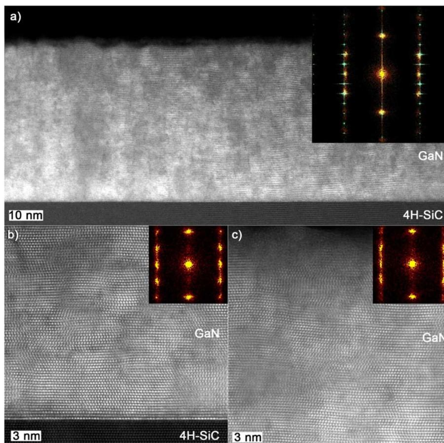
**Fig. 4** Overview of the STEM-HAADF image from the GaN film with a thickness of approximately 60 nm on 4H-SiC. HR-STEM-HAADF image of the film–substrate interface and (c) top part of the film. The FFT patterns are shown as insets in (a–c) with orange as GaN and cyan as the 4H-SiC substrate. Reprinted from Rouf *et al.*<sup>37</sup> under a CC-BY license.
